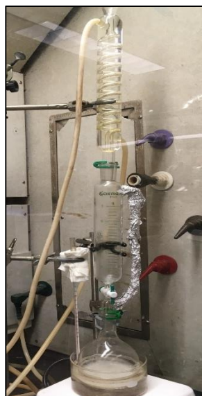
Figure 26: Pressure equalizer and condenser arrangement for drying THF.
