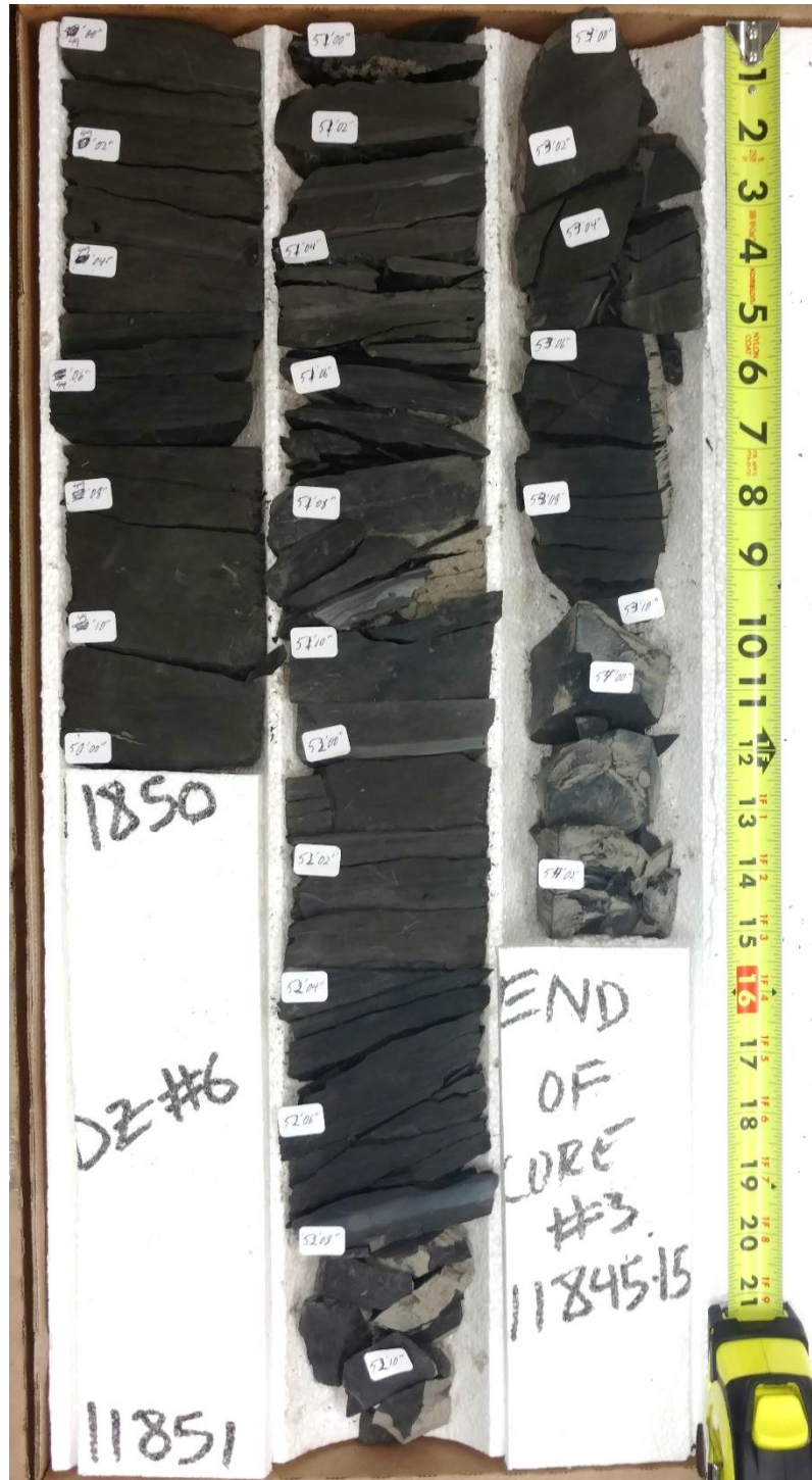
Figure 22. Clay-rich base of Velma core. Depth interval 11,849'-11,854'11".
