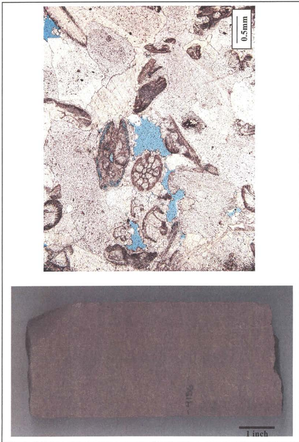
Figure 18. Core photograph and photomicrograph of the Frisco Formation mud mound/bioherm facies. Baxter #1 well. Depth 4,156 feet.
