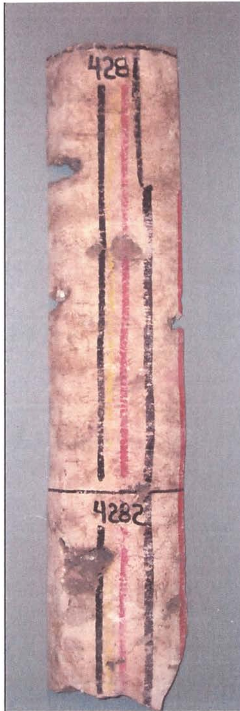
Figure 29. Photograph of core showing large vugs that reflect the extent of focused-flow karstification. Typical in Silurian section of the Hunton Group. The Frisco is generally karstified by more diffuse-flow type dissolution that results in moldic porosity. Ponkilla #1 well. Depth 4,282 feet.
