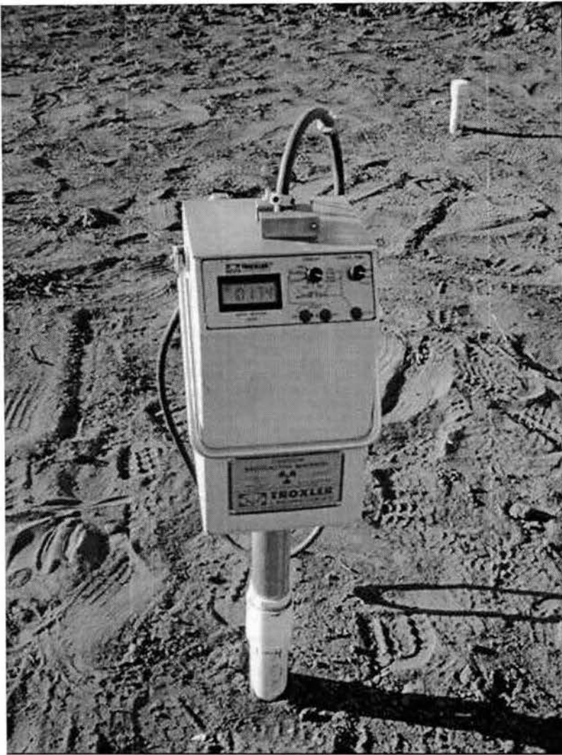
Figure 7. Neutron probe measurement of volumetric soil moisture
