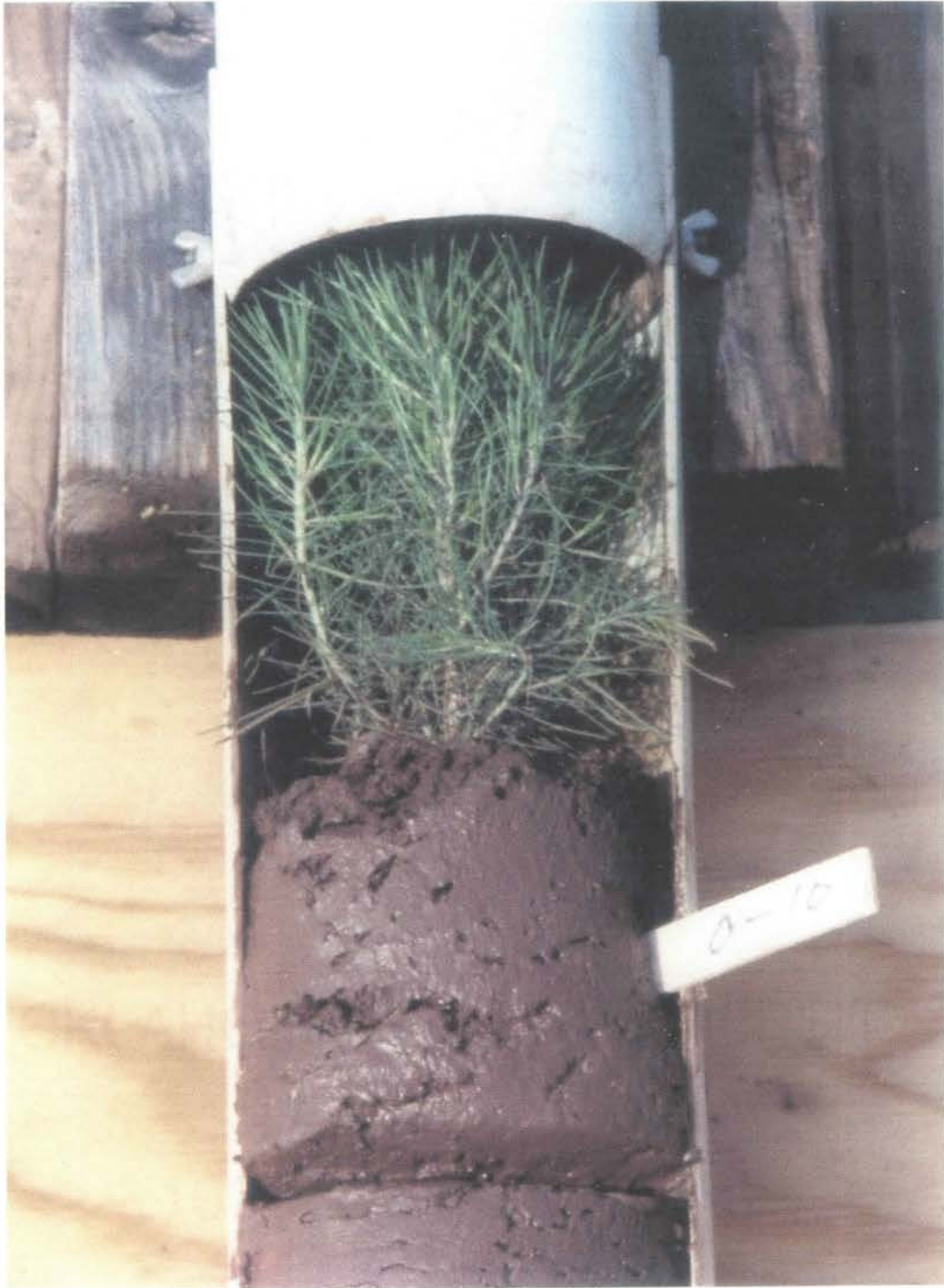
Fig. 4. Soil core extracted from the PVC pipe showing 0 to 10 cm profile and seedlings.
