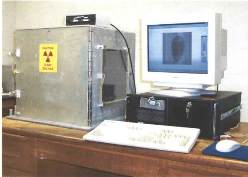
Figure D.1 The X-ray imaging system showing shielded box, X-ray tube controller, computer, and monitor.
