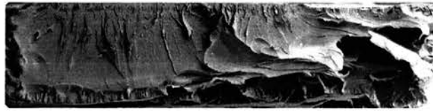
(A) \sigma_a = 36.5 \text{ Mpa} , \log(N_f) = 3.25
