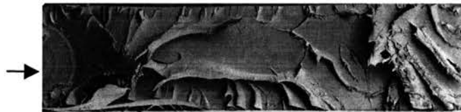
(C) \sigma_a = 14\text{Mpa} , \log(N_f) = 3.5
