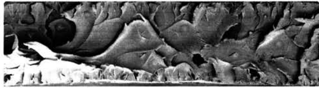
(A) \sigma_a = 19.5\text{Mpa} , \log(N_f) = 2.85
