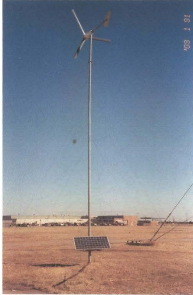
Figure 2. Bergey hybrid system: wind turbine with solar battery (Photo was taken by E. Ermilova on January, 31 in Bergey Wind Industry, Norman, OK).
