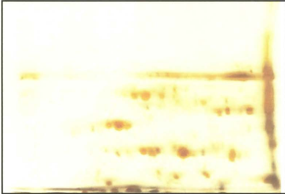
Figure 3. TCA/Acetone extraction of wheat leaves, followed by resuspension into urea buffer (1 \mu g powdered extract /30 \mu l resolubilization solution; loaded 125 \mu l of solution onto an 11% gel) using only a warm water bath to aid in resolubilization.
