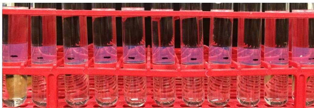
Figure 19: Sample salinity scan for 0.054M BCl and toluene for salinities 4.0, 4.6, 4.7, 4.8, 4.9, 5.0, 5.1, 5.2, 5.3, 5.4, and 6.0 g NaCl/100 mL H 2 O
