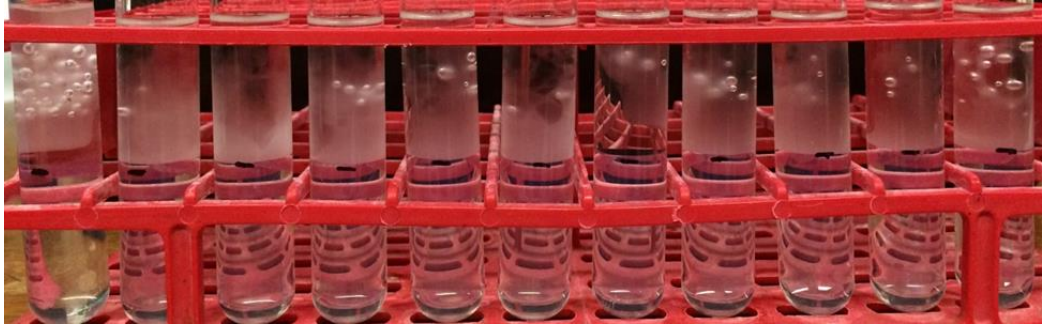
Figure 20: Sample salinity scan for 0.01M BCl and hexane for salinities 10.5, 11.3, 11.4, 11.5, 11.6, 11.7, 11.8, 11.9, 12.0, 12.1, and 13.0 g NaCl/100 mL H 2 O
