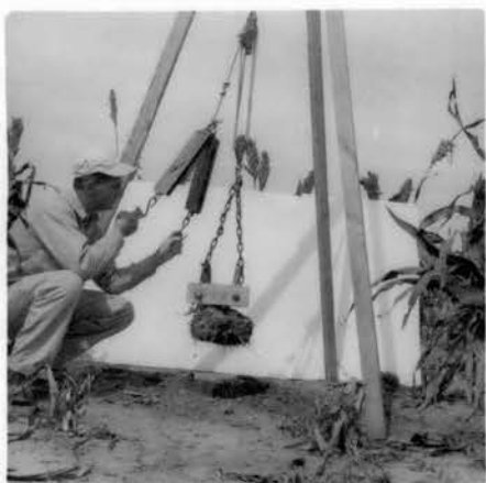
Fig. 7 - Plant pulling device used to apply and measure force necessary to uproot hills of sorghum varieties.
