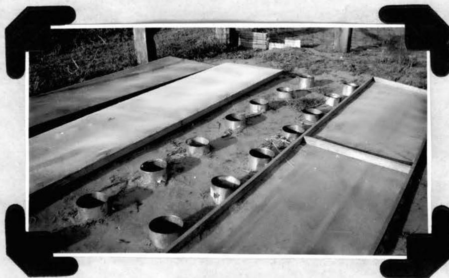
Figure 2.--Sunken cages used in life history work. The screen frames were used to cover cages at night.
