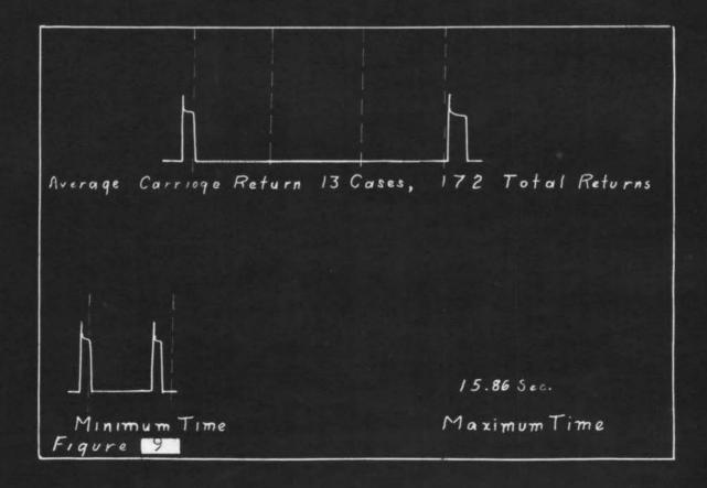
Shifting requires two operations, depressing and releasing the shift key, and making the stroke. A stroke is shown by a variation in the recorded line. Striking and releasing the shift key would move the second pen marking the period of shift key depression with a line over the graph indicating the stroke. Its deviation to the right or left indicates whether the stroke was being made too soon or too late for the letter to be exactly on the line of writing.
