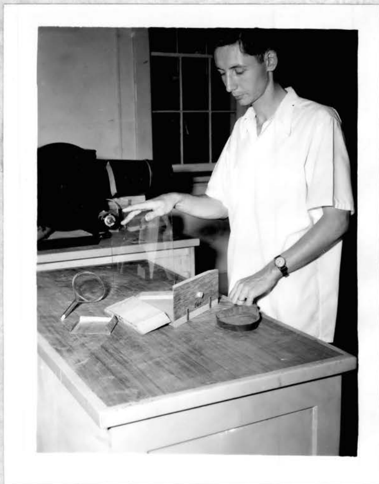
Plate 1 - A test box with glass cover and rubber band (to hold sides tightly together). Glass funnel and metal slide are also shown.
