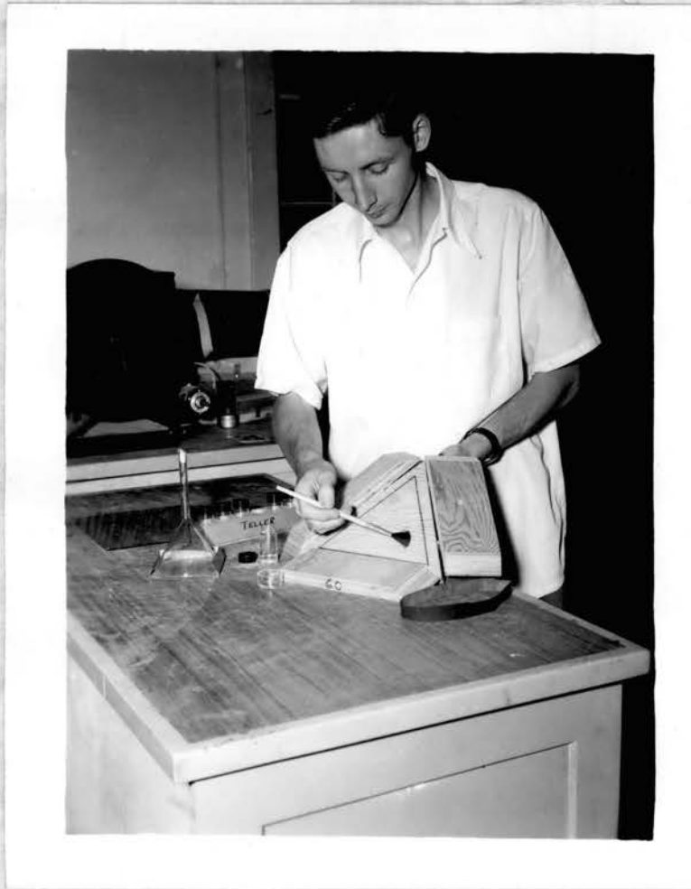
Plate 3 - Method of painting 4 ml. of oil solution on a test box.
