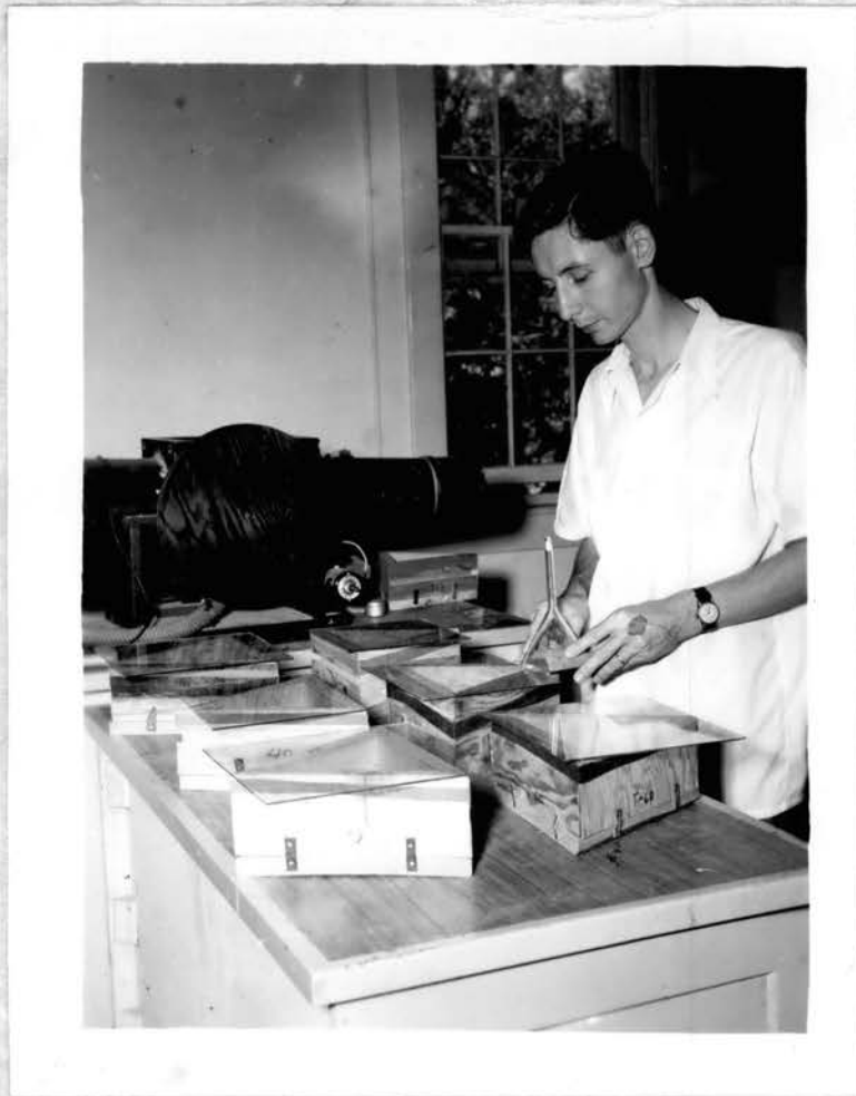
Plate 2 - Method of introducing flies into test boxes.
