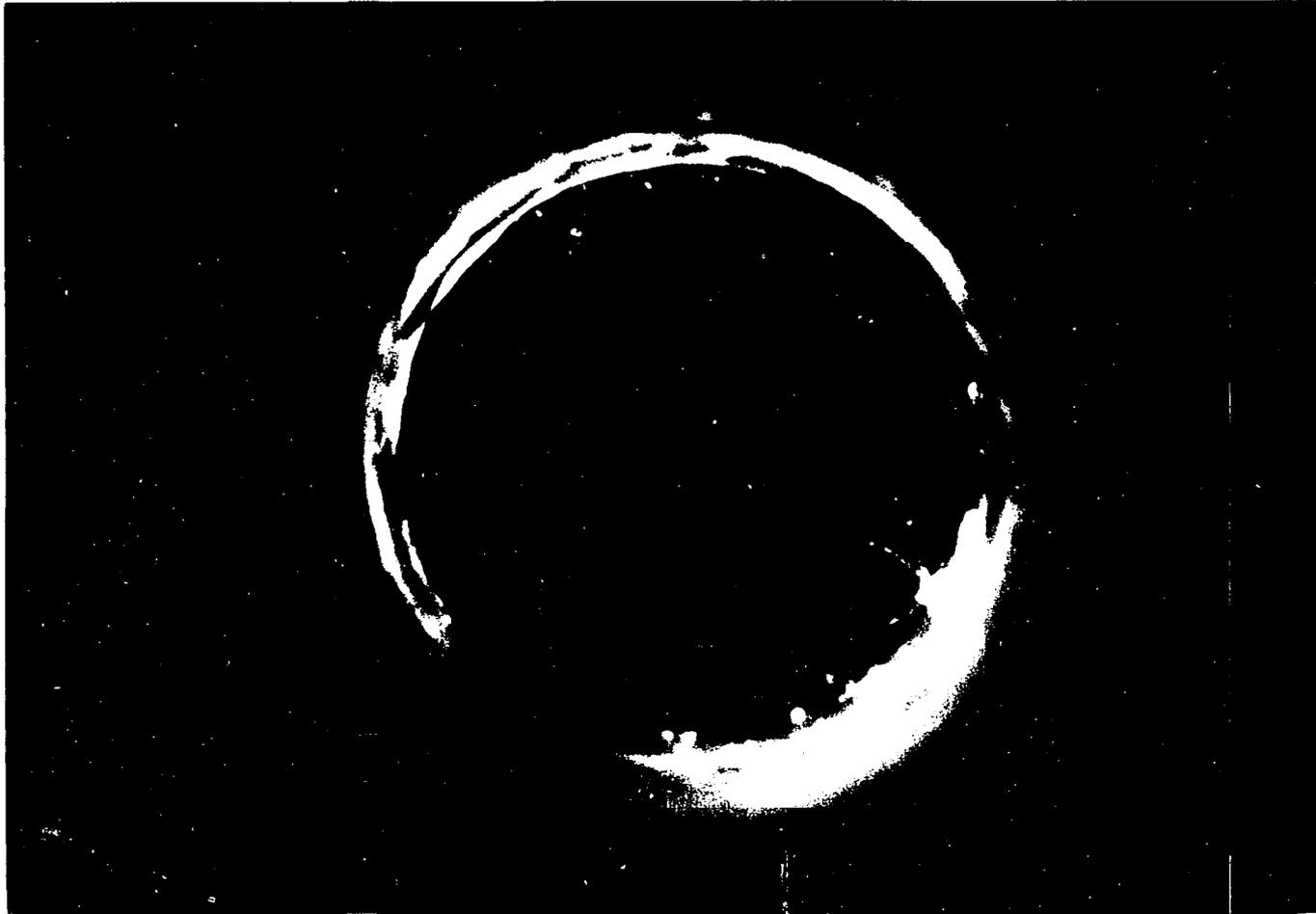
Figure 45b. Axial Photograph Showing the Interchange Between Liquid Film on the Wall and the Droplets in the Core Region for Flow Condition 460, Slide No. 35.
