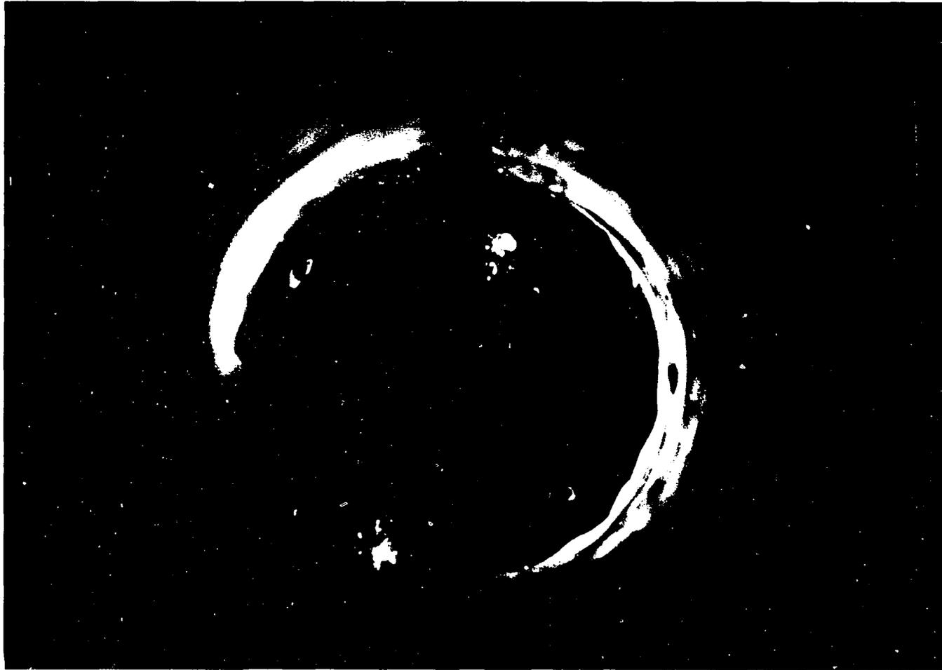
Figure 45a. Axial Photograph Showing the Interchange Between Liquid Film on the Wall and the Droplets in the Core Region for Flow Condition 360, Slide No. 19.
