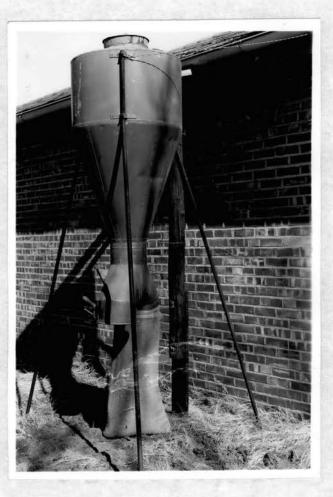
Figure 3. Hammer Mill Hopper For Collecting Dust and Chaff.
