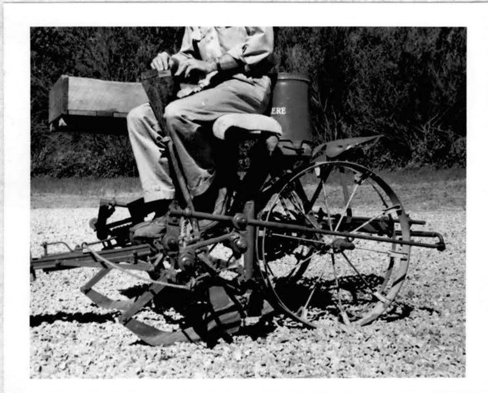
Figure 1.-- A two-row corn planter modified for planting experimental plots.
