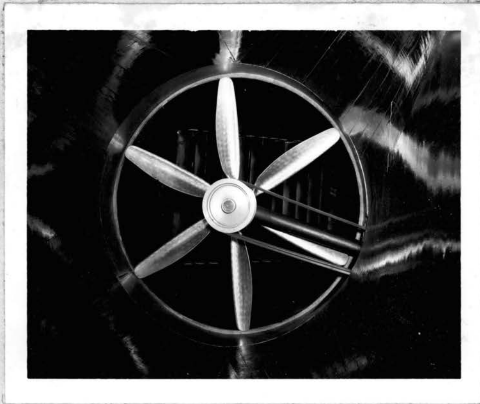
Fig. 6. Propeller Section of Tunnel.
