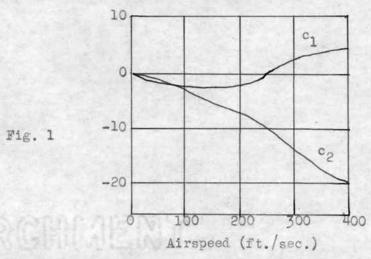
The curve c<sub>1</sub> of Fig. 1 represents the damping factor of one oscillatory constituent which is damped for all speeds less than 240 ft/sec. and grows indefinitely laxys for all speeds greater than this value, while c<sub>2</sub> of the second constituent remains damped for all speeds.
