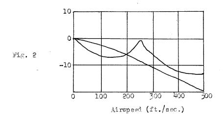
Both of the constituents of the oscillation in Fig. 2 remain damped throughout the range covered by the diagram, however there is a very small margin of stability in the vicinity of 250 ft/sec.
