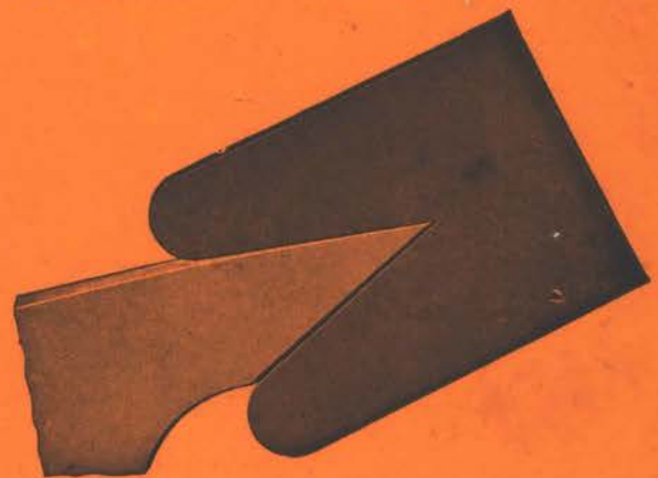
Tooth Gauge by which to file and regulate the shape of teeth.
