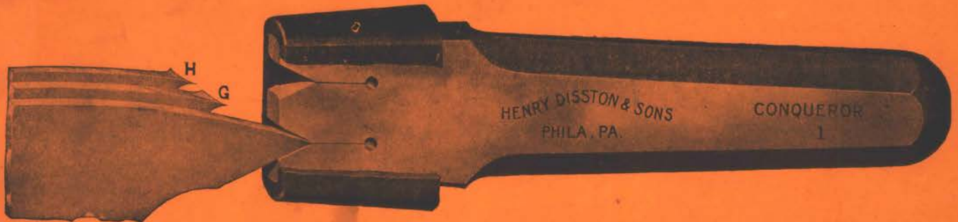
Conqueror Swage, showing angle at which die should be placed on tooth. "H" shows shape of tooth after using convex die. "G" shows finished edge of tooth after using straight die.
