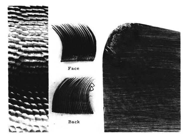
10X PHOTOMACROGRAPH OF WORK SURFACE, CHIP, & TOOL SAE 1020 STEEL
