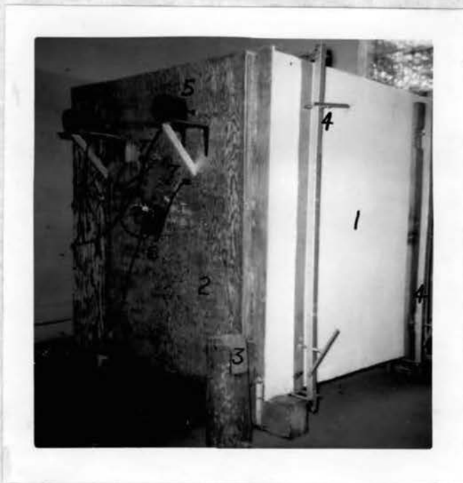
Figure 3 - TEST WALL AND GUARDED HOT BOX
