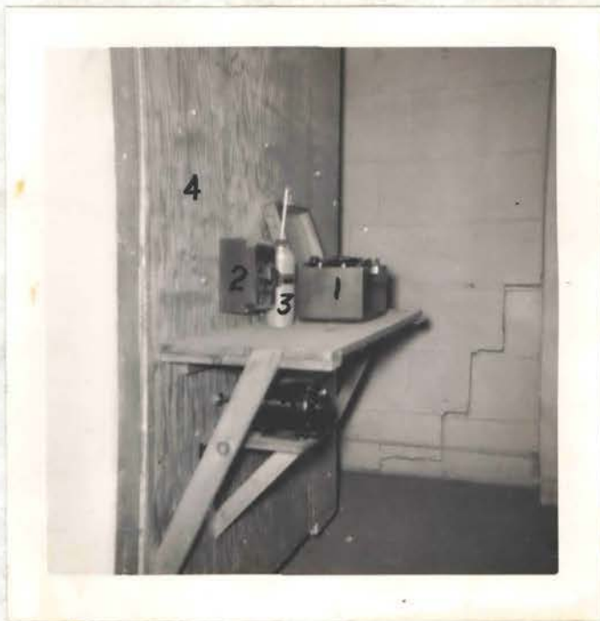
Figure 5 - TEST INSTRUMENTS OF GUARDED HOT BOX
