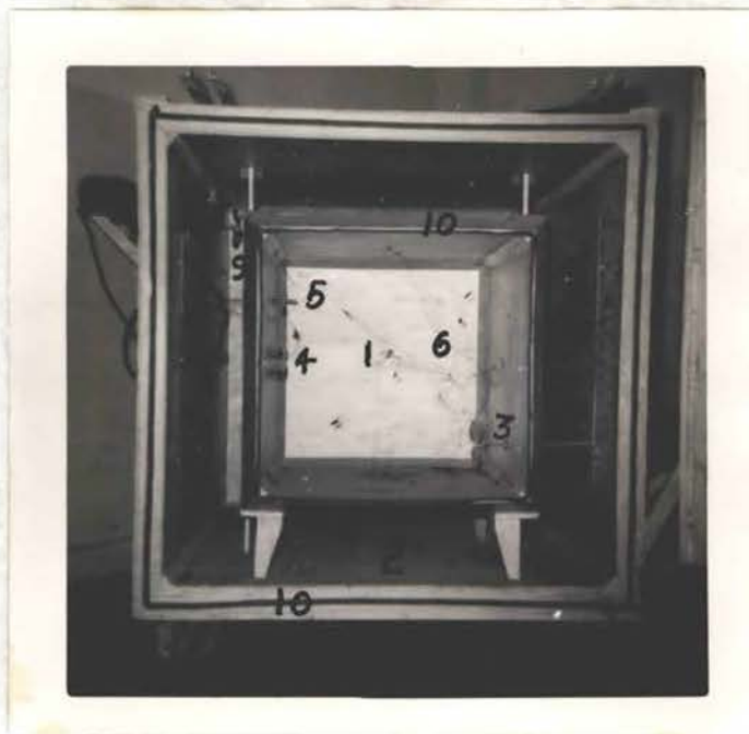
Figure 4 - INTERIOR OF GUARDED HOT BOX
