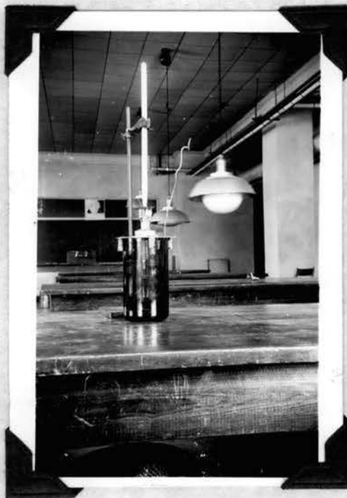
Fig. 20 Beckman thermometer set up for determining osmotic pressure.
