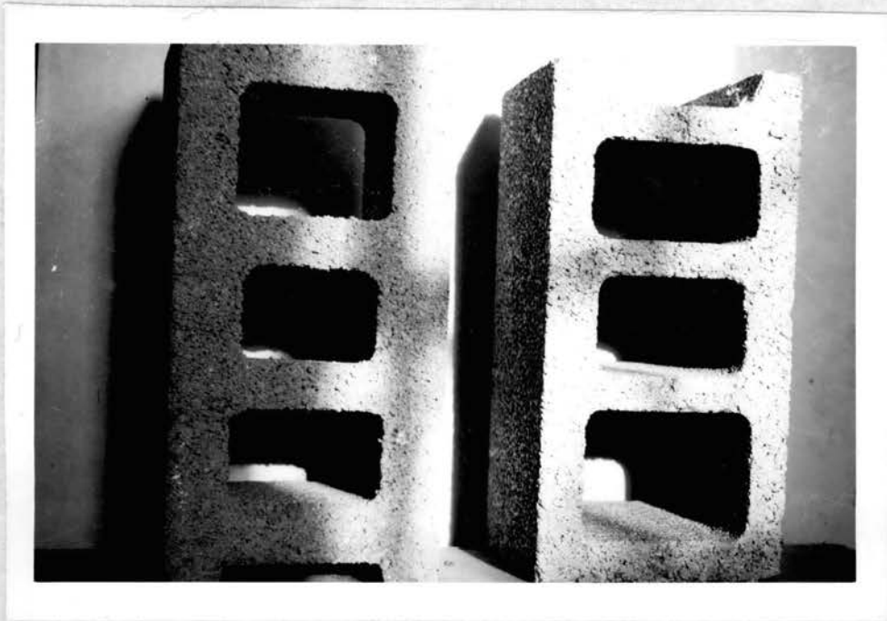
Fig. 8 - Opposite Core Ends of Expanded Shale Aggregate Concrete Block Used in Temperature Controlled Shelter.
