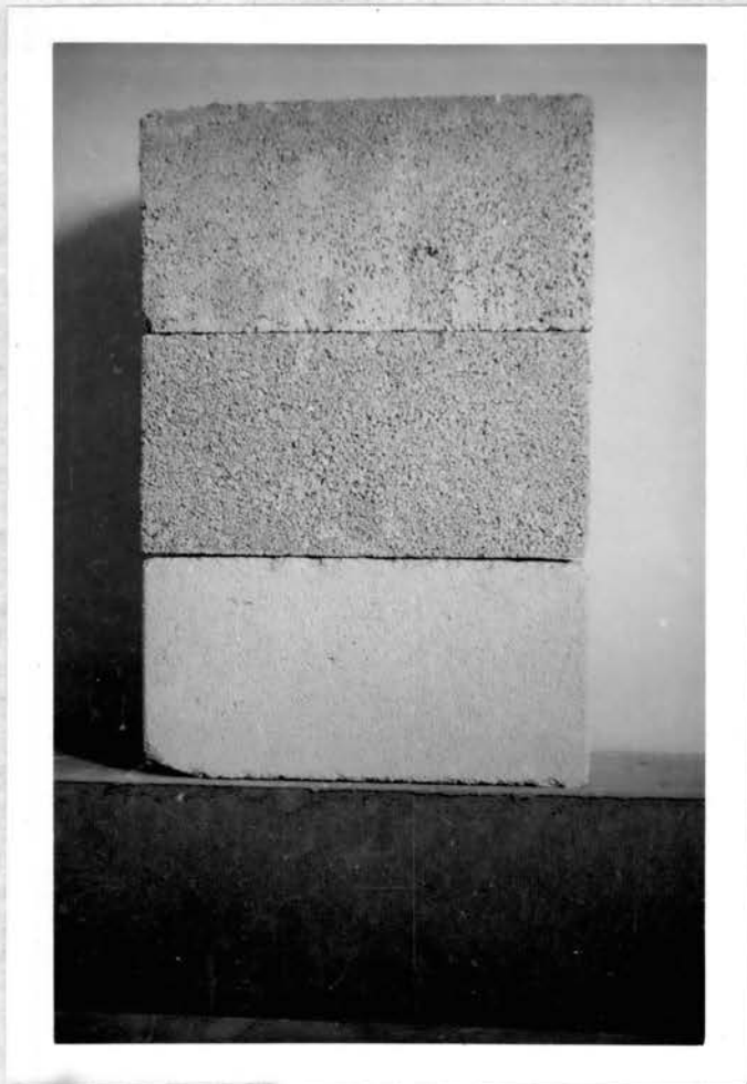
Fig. 8 - Opposite Core Ends of Expanded Shale Aggregate Concrete Block Used in Temperature Controlled Shelter.
