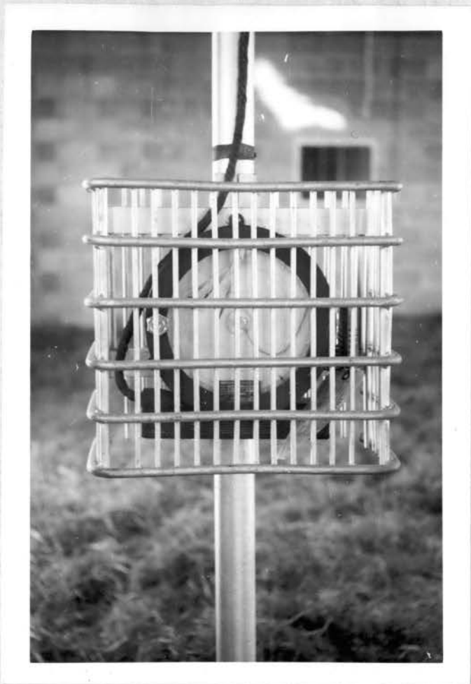
Fig. 10 - Dry Bulb Temperature and Relative Humidity Recorder Used in Temperature Controlled Shelter.
