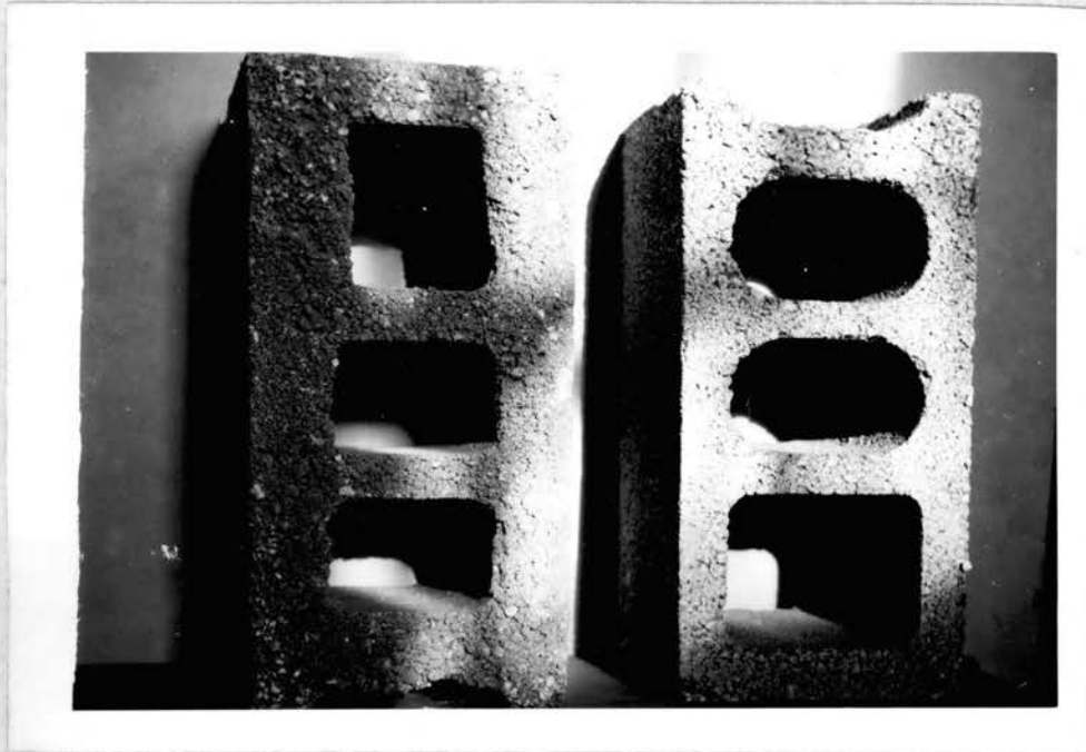
Fig. 6 - Opposite Core Ends of Pumice Aggregate Concrete Used in Walls of Temperature - Controlled Shelter.
