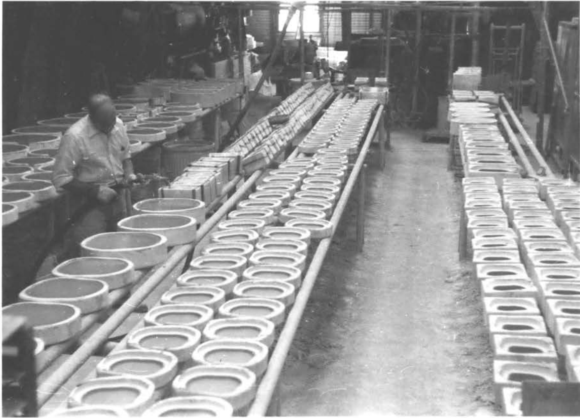
Filling the molds with slip.
