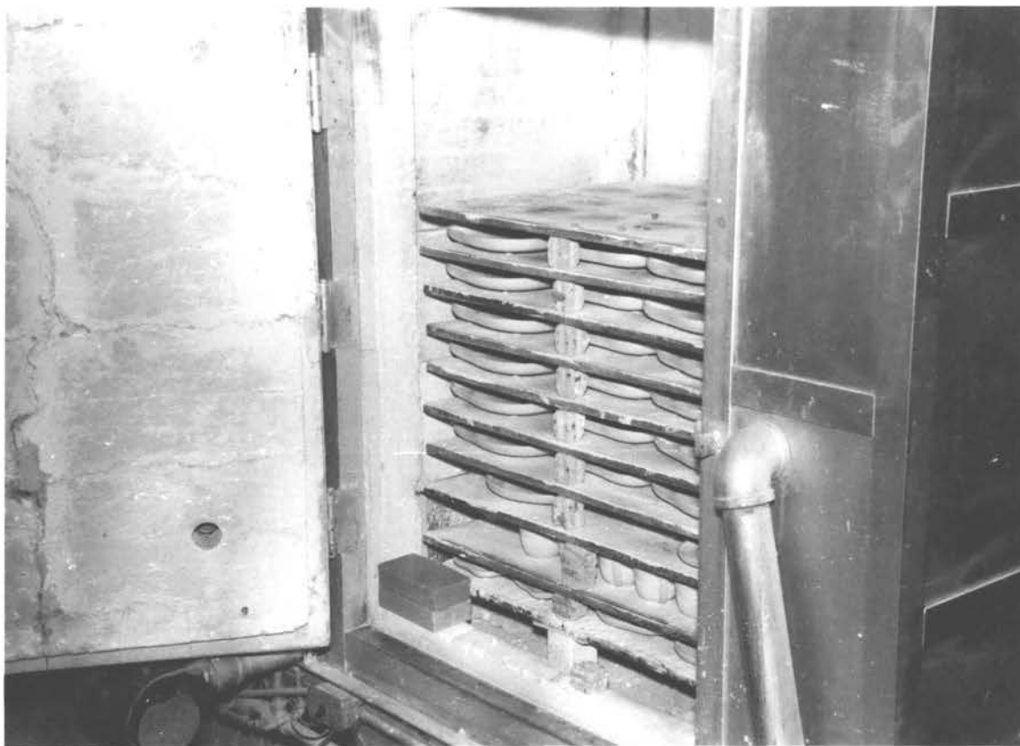
This is a glaze kiln partly filled.
