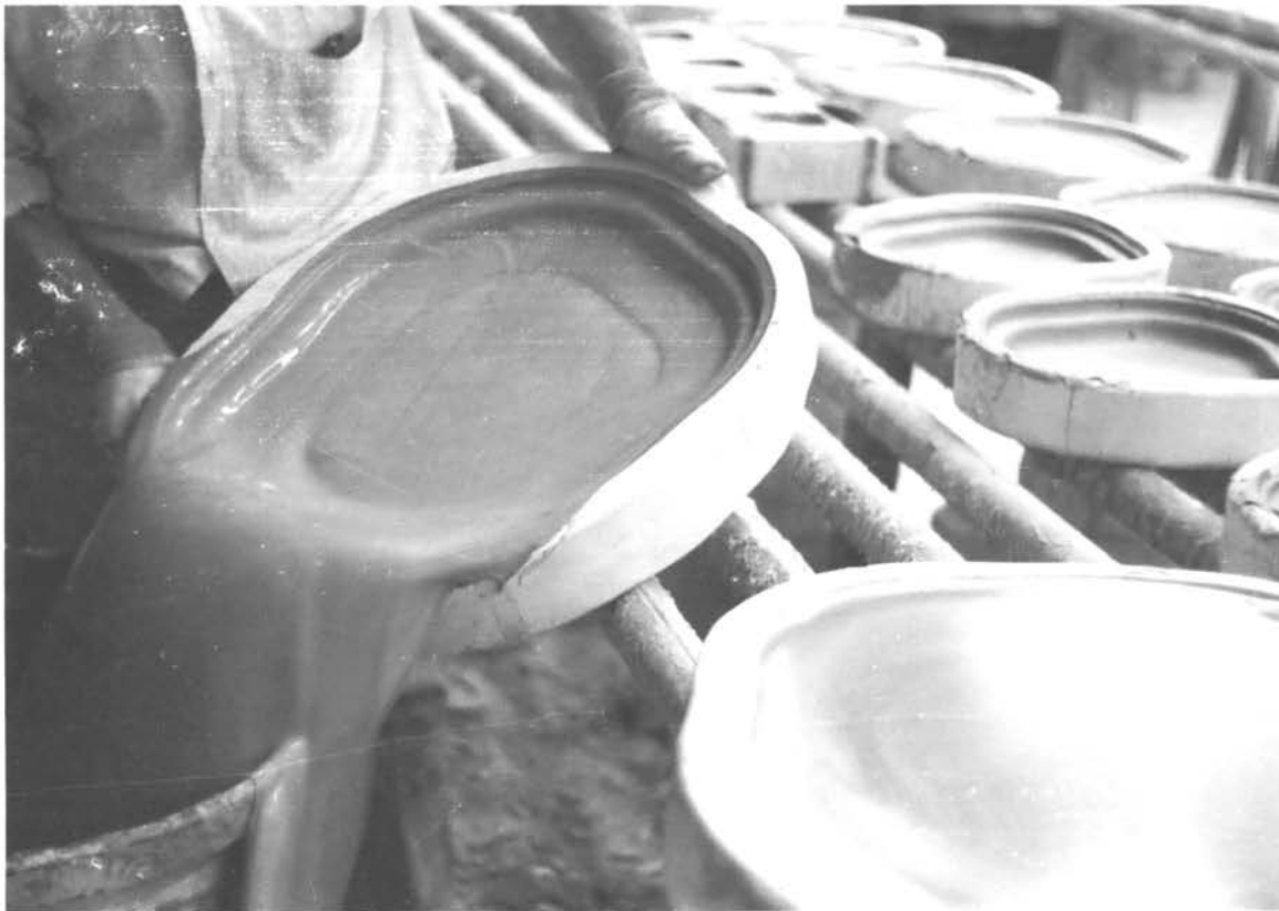
Pouring excess slip from molds.
