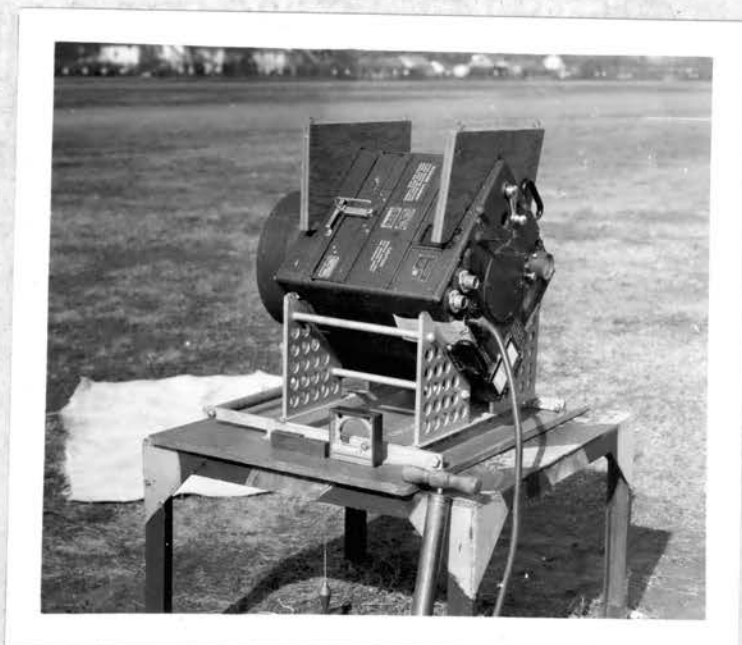
T-5 camera on camera platform. Film magazine in place. Note camera sights, vacuum pump, and cloth on ground.
