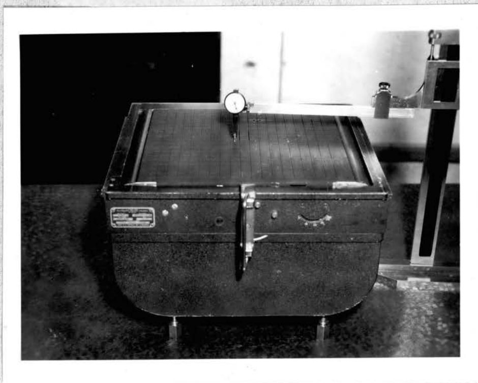
Magazine from T-5 camera. The vacuum back is being measured for flatness with height gage and dial indicator. Magazine rests on small jacks which rest on surface plate.
