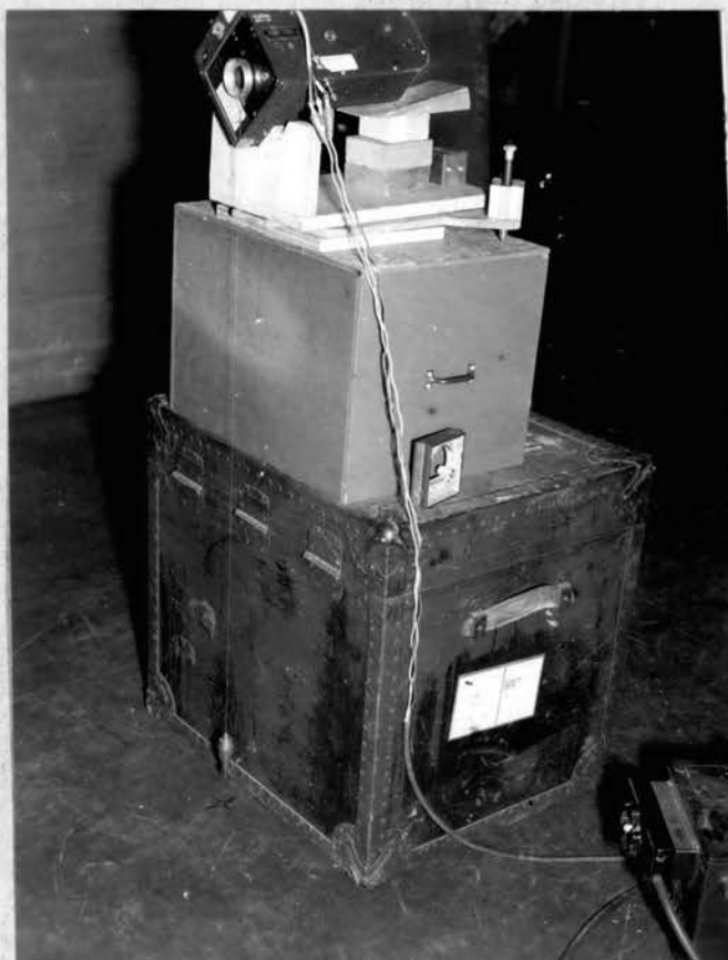
A. 35 mm Type O-15 Radar Recording Camera over reference point on indoor calibration range
