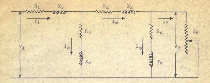
Figure 1. The exact equivalent circuit for the singlephase induction motor.
