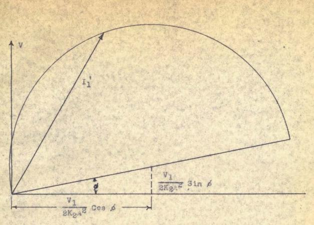
Figure 3. The circle diagram representing the locus of the rotor current of a single-phase induction motor.
