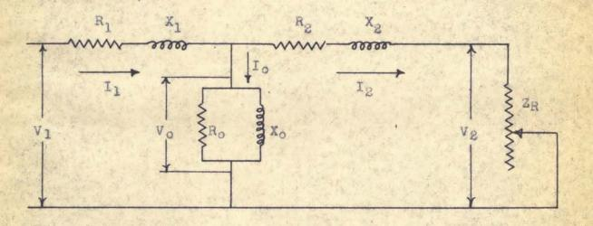
Figure 2. The approximate equivalent circuit for the single-phase induction motor.
