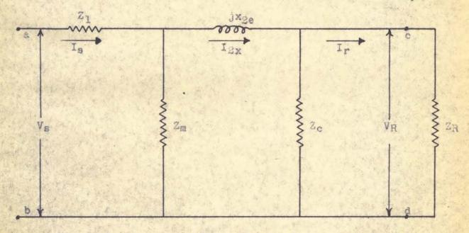
Figure 6. An equivalent circuit for a single-phase motor.
