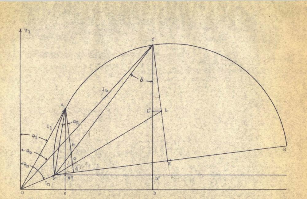
Figure 7. Circle diagram of a single-phase induction motor used to obtain the calculation sheet.
