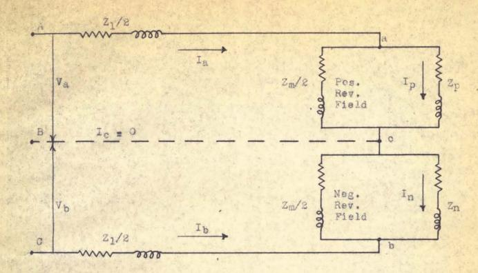
Figure 5. Equivalent-rotating-field circuit diagram of a single-phase motor.
