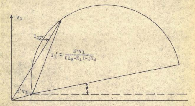
Figure 4. The circle diagram representing the locus of the stater current of a single-phase induction motor.
