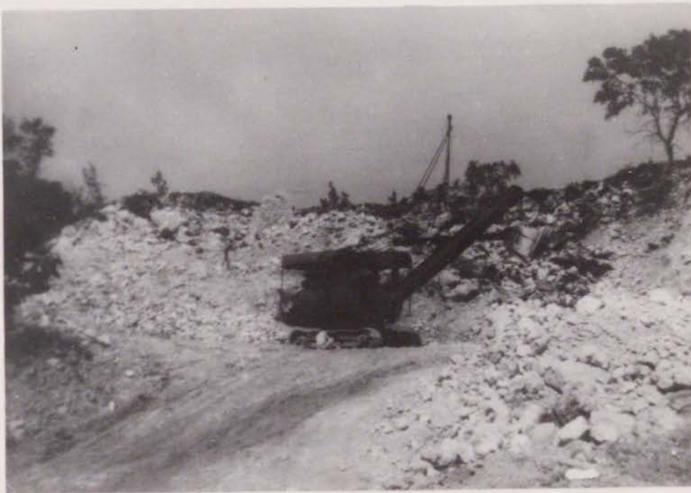
Fig. 19b. Excavator and rig of the Choctaw Lime Company. The rig (on top of cliff) digs a forty foot hole for the charge. The excavator loads the lime boulders into dump trucks for the crusher.
