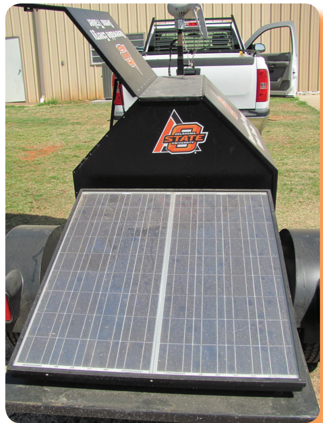
Picture above: Solar photovoltaic panels on the BAE renewable energy demo trailer.
