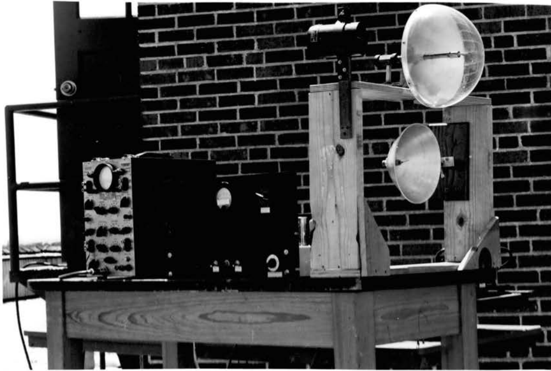
Figure 4. Transmitting and Receiving Antennas
