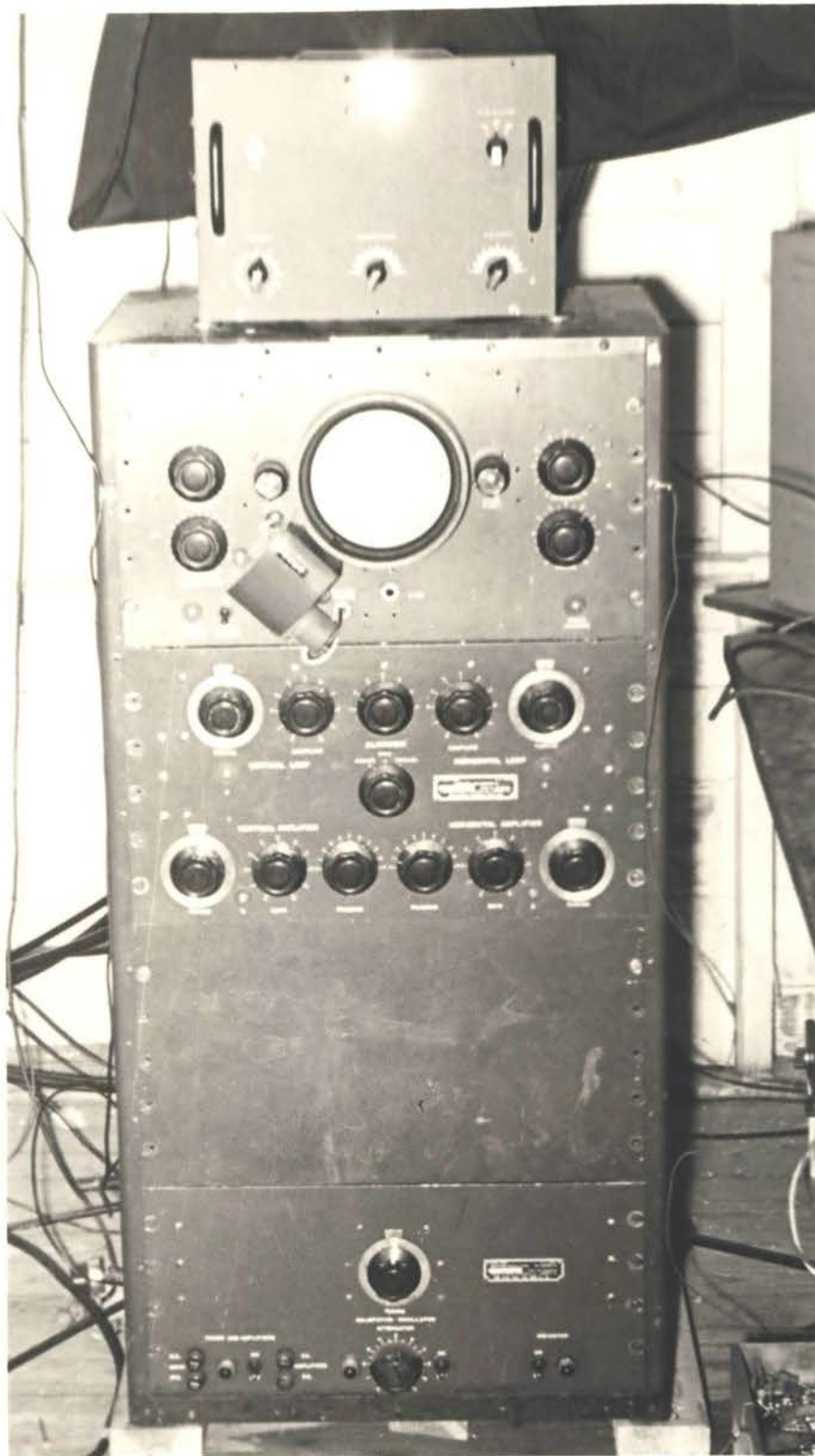
Figure 13. Front view of the spheric direction finder and ambiguity eliminator.
