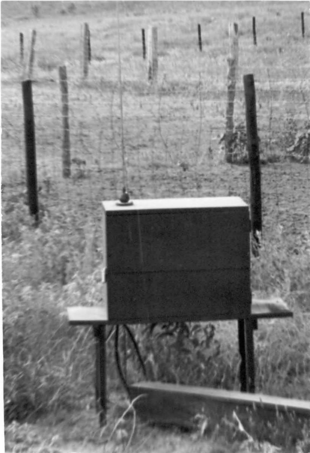
Figure 4. Remote installation of the antenna to coaxial line cathode follower.
