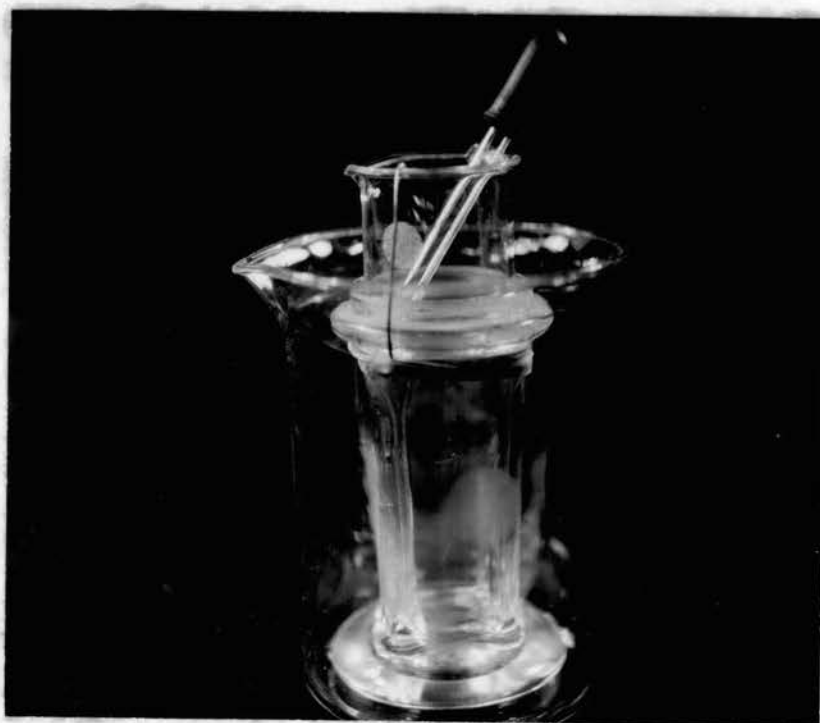
Fig. 1. Apparatus used for melting the emulsion prior to coating slides.
