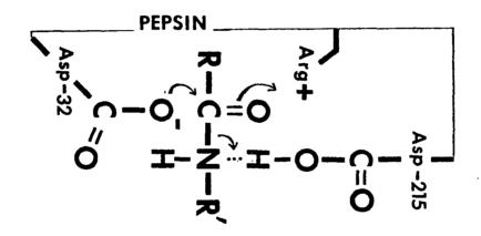
directly involved in catalysis. This mechanism is very similar to that proposed independently by Hunkapiller and Richards (65).
