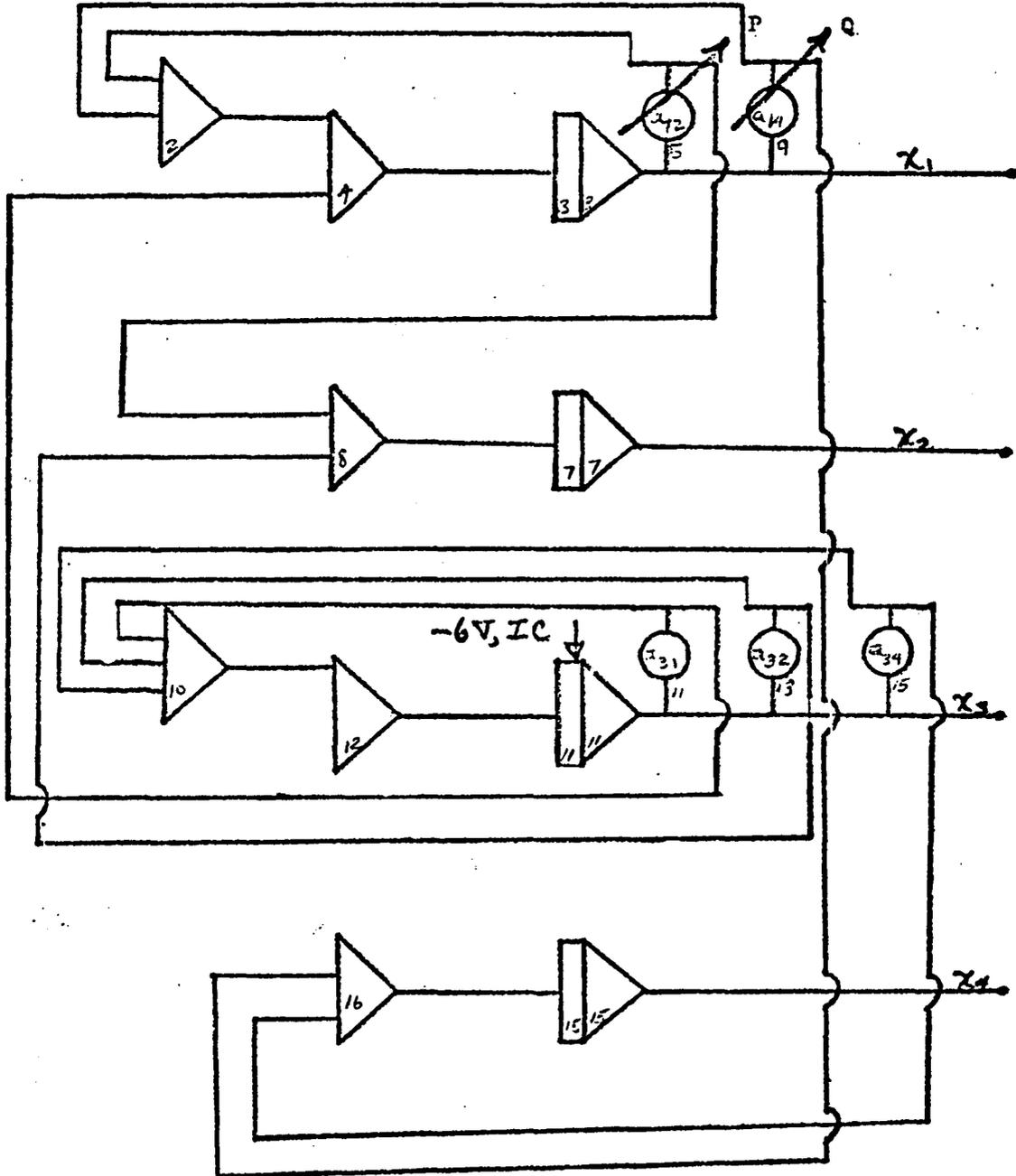
Figure 25. Complete Analog Computer Program
