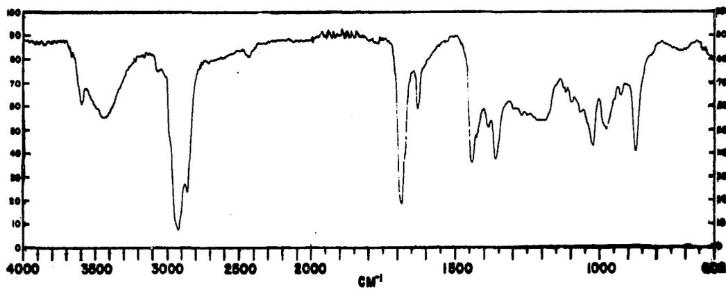
IR Spectrum (CHCl<sub>3</sub>) of B-3 (30)
