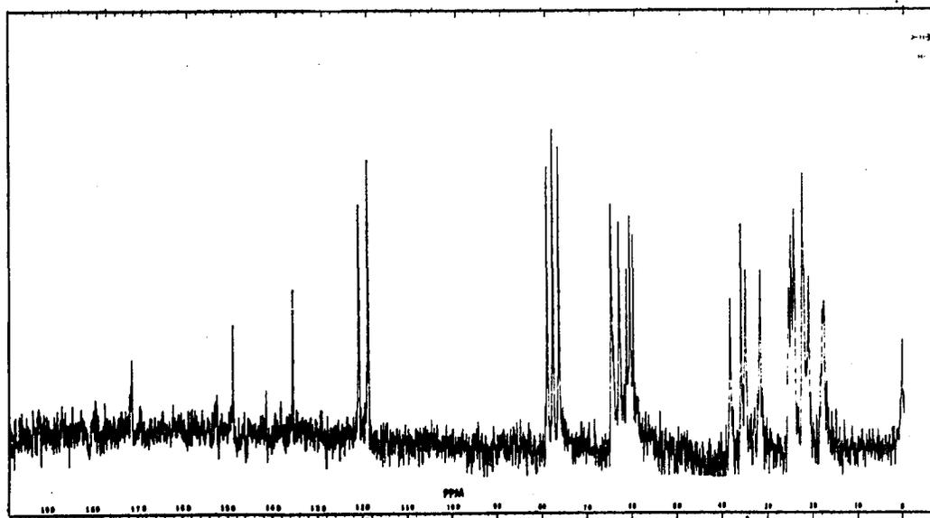
25.2 MHz Proton-Decoupled CMR Spectrum ( $\text{CDCl}_3$ )
