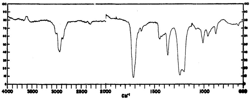
IR Spectrum (CHCl<sub>3</sub>) of B-3 Diacetate (31)
