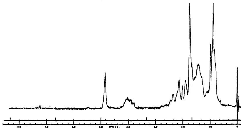
60 MHz PMR Spectrum (CDCl<sub>3</sub>) of 30
