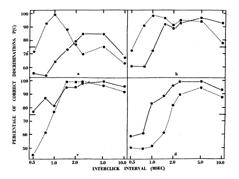
Figure 15.--Percentage of correct discriminations by Subject 5, as a function of the interclick interval, for four values of the interclick intensity ratio. Each section of the figure represents performance for a single value of the interclick intensity ratio: a) 3 dB; b) 6 dB; c) 12 dB; and d) 24 dB. The level of signal presentation was either 75 dB SL (------).
