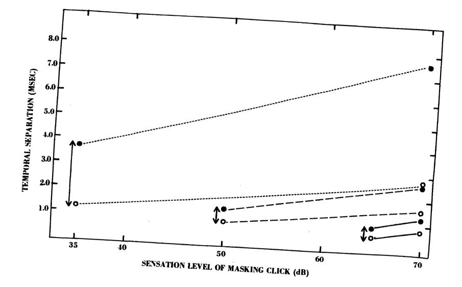
detection of the less intense click in the forward-and backward-masking conditions is smallest). It is also apparent from Figure 3 that the asymmetry at a given interclick intensity ratio (such as that for  $\Delta I$  of 20 dB, indicated by the arrow) is reduced as the intensity of the more intense click is increased.
