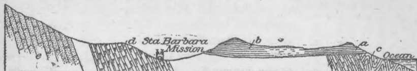
FIG. 39.—Section from the Pacific to the Santa Inez chain, at Santa Barbara. Distance about 3 miles. a, b, Pliocene and Pleistocene strata; c, bituminous slate, much contorted; d, bituminous slates and fine grained sandstones; e, sandstone, dipping south.
