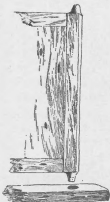
FIG. 76. Wooden pivot hinges of a Zuñi door.
