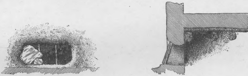
FIG. 89. Sloping selenite window at base of Zuñi wall on upper terrace.
