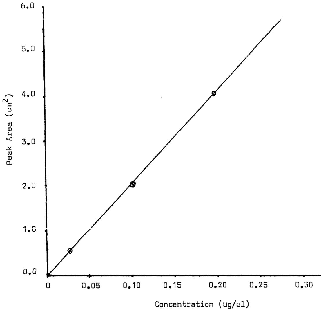
Figure 18.--Plot of concentration against peak area (at  $200^\circ\text{C}$ ) for pyrene.
