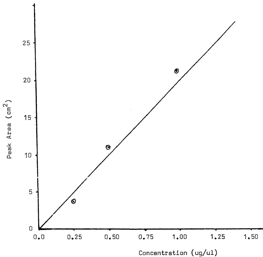
Plot of Concentration against Peak Area (at 200°C) for o-Phenylene pyrene.
