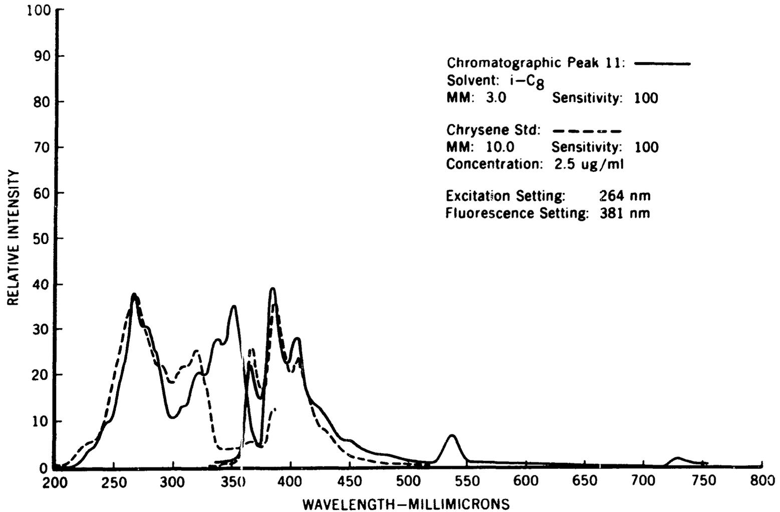
Excitation and Fluorescence Spectra of Chromatographic Peak 11 from SRF Carbon Black Extract and Chrysene.
