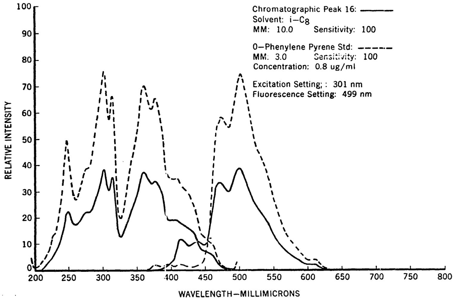
Excitation and Fluorescence Spectra of Chromatographic Peak 16 from SRF Carbon Black and
