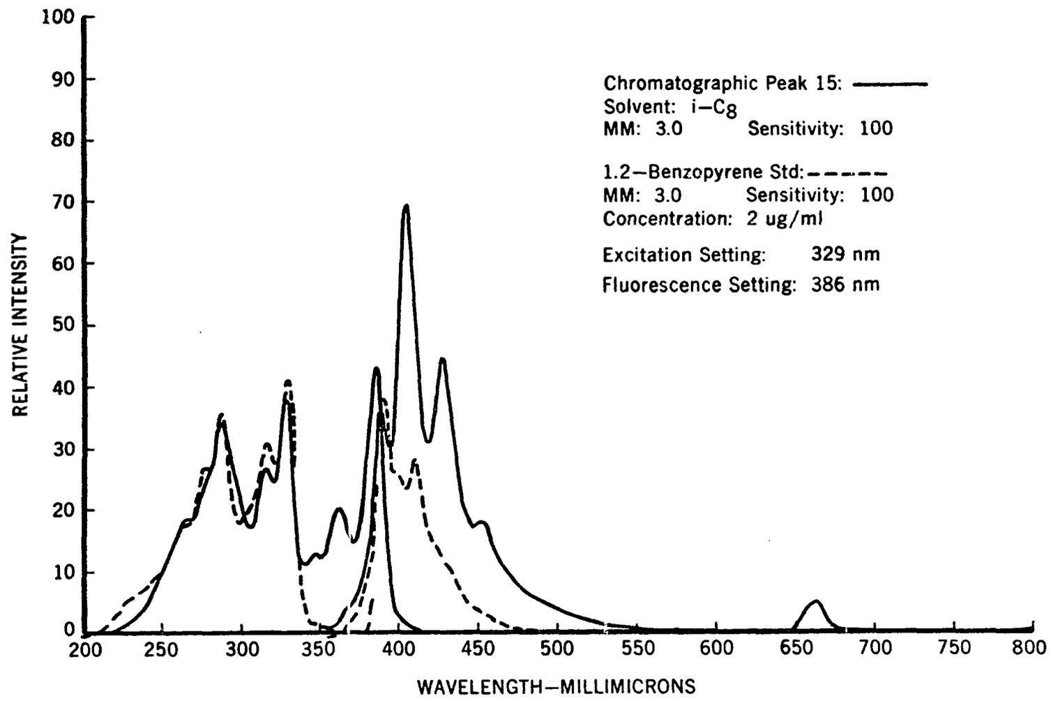
Figure 13.-- Excitation and Fluorescence Spectra of Chromatographic Peak 15 from SRF Carbon Black Extract and 1,2-benzopyrene.
