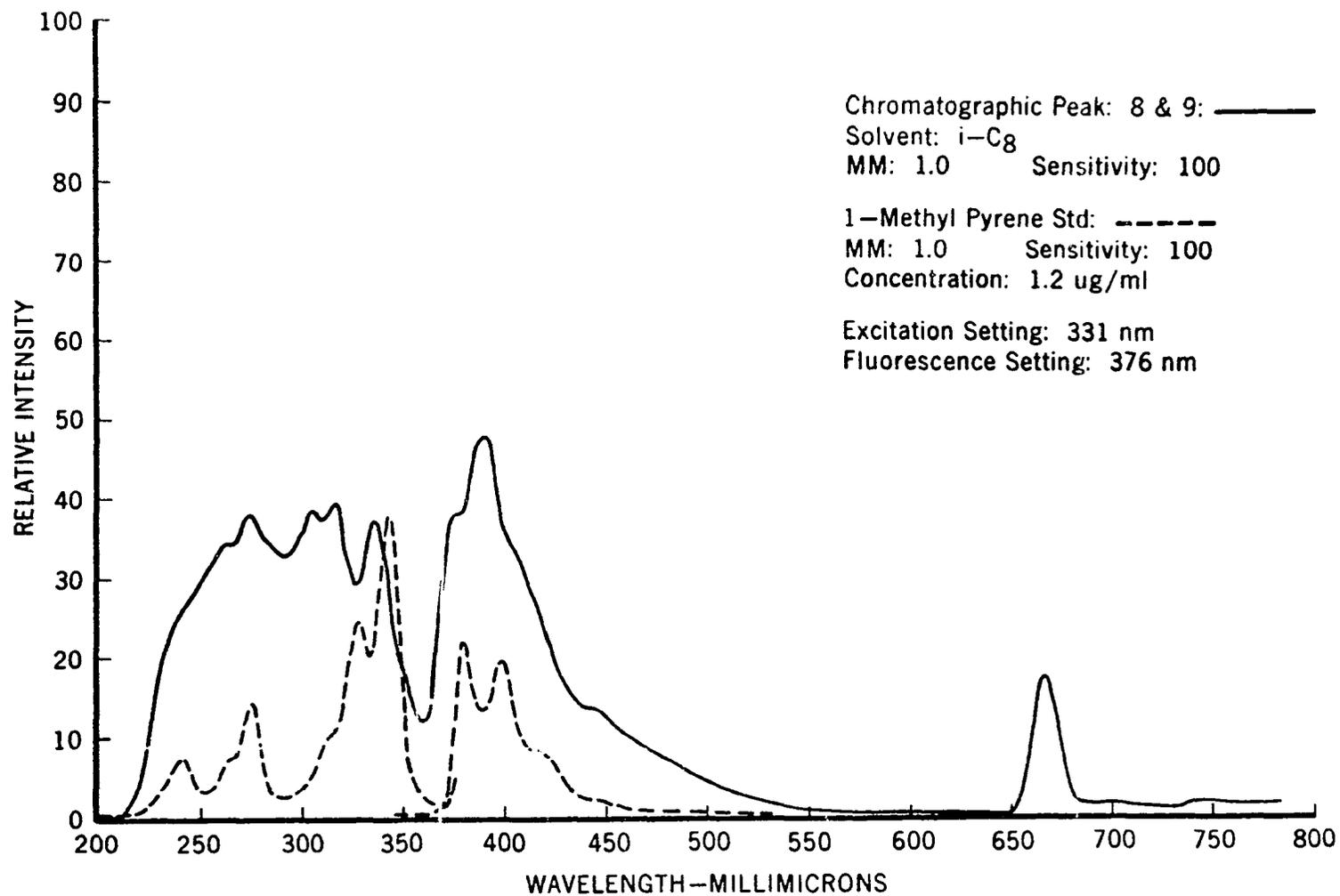
Excitation and Fluorescence Spectra of Chromatographic Peak 8 & 9 from SRF Carbon Black Extract and 1-Methyl Pyrene.
