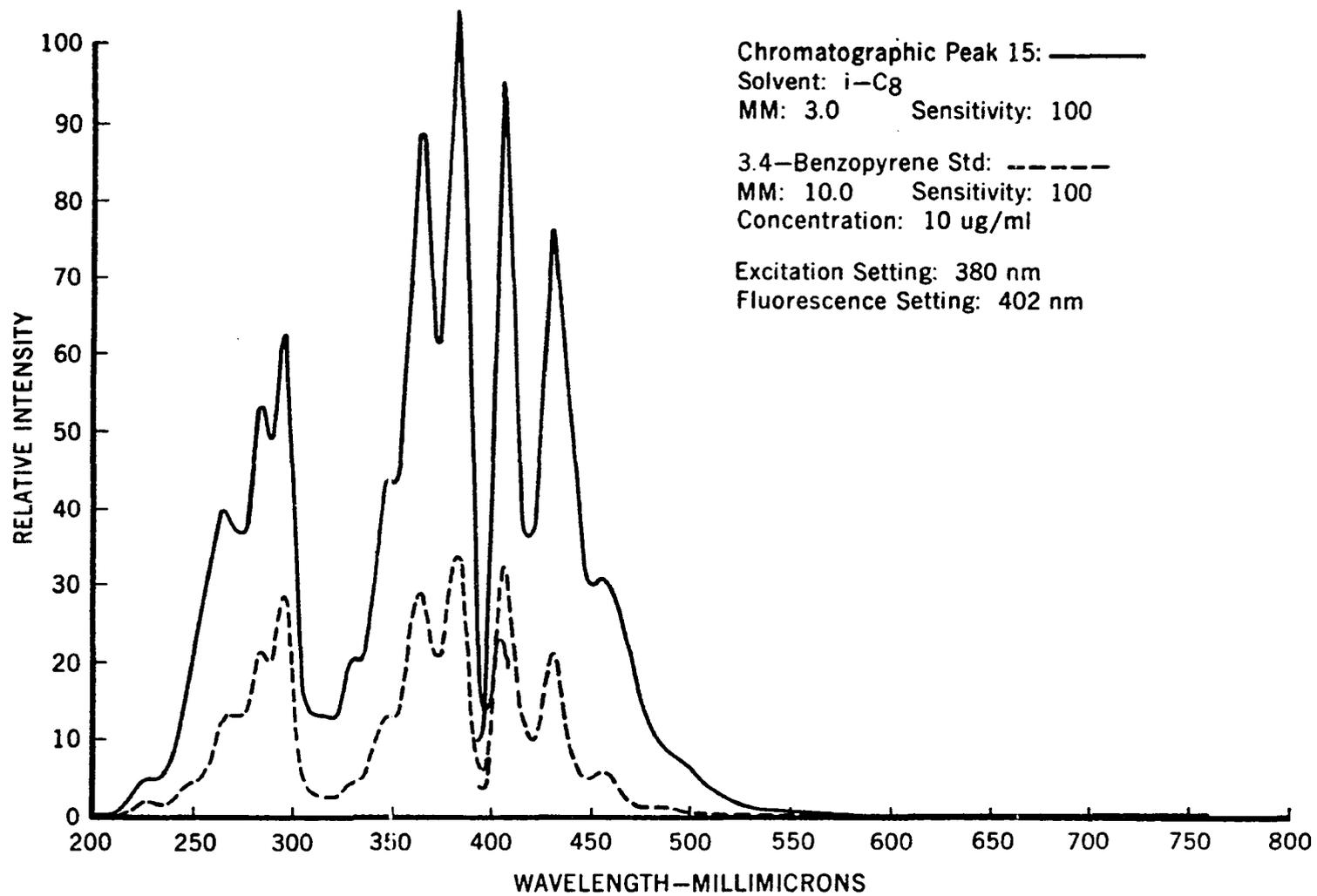
Figure 14. --Excitation and Fluorescence Spectra of Chromatographic Peak 15 from SRF Carbon Black Extract and 3.4-benzopyrene.
