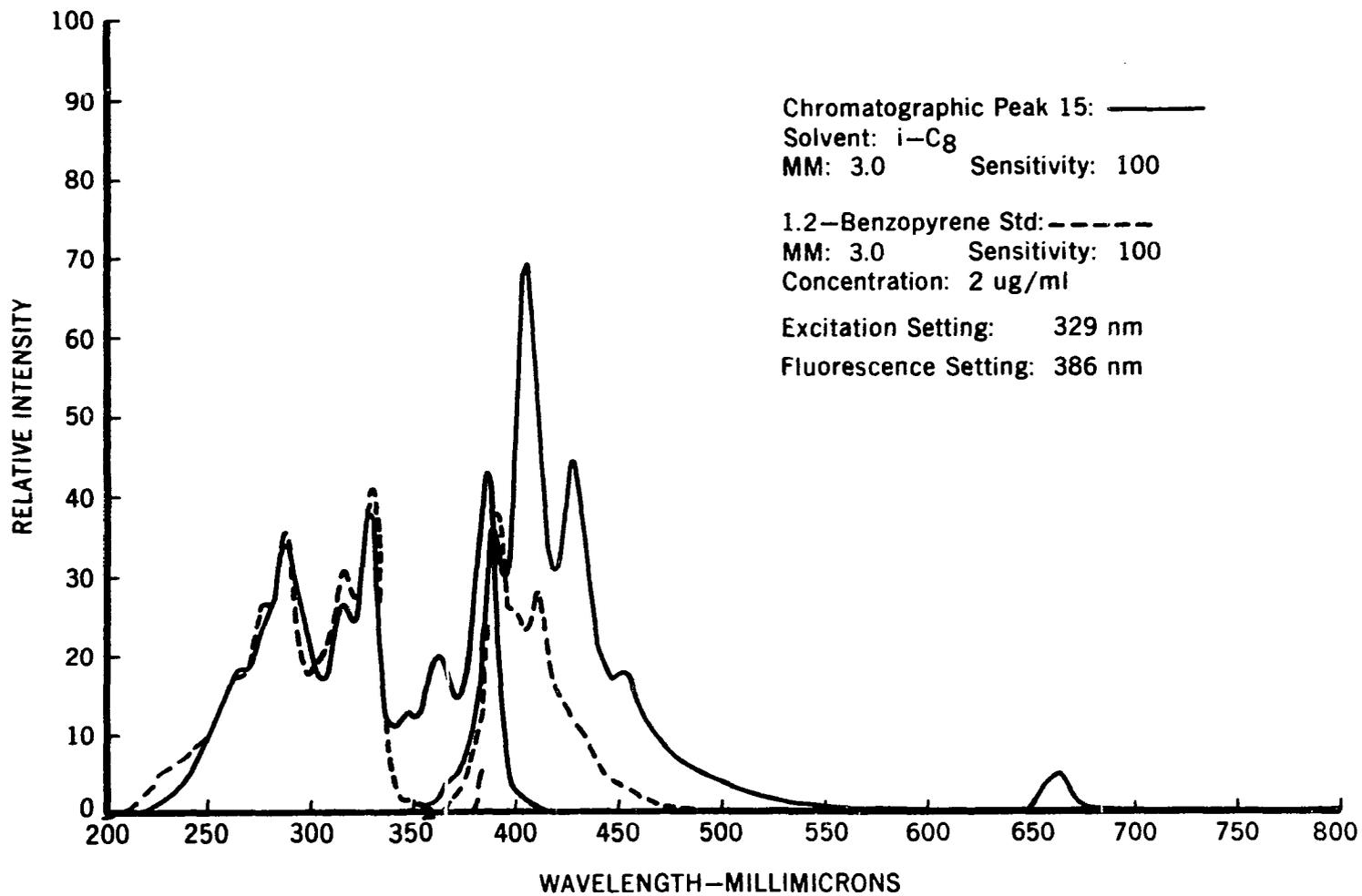
Excitation and Fluorescence Spectra of Chromatographic Peak 15 from SRF Carbon Black Extract and 1.2-benzopyrene.
