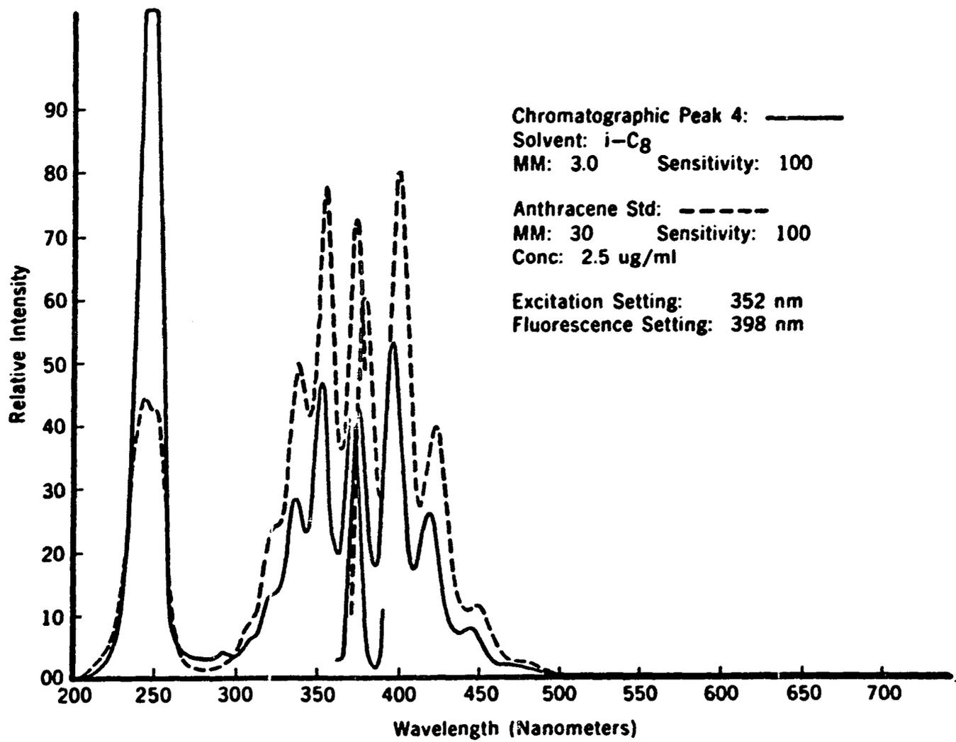
Figure 2. -- Excitation & Fluorescence Spectra of Chromatographic Peak 4 from Carbon Black Extract and Anthracene in *i*-C<sub>8</sub>.
