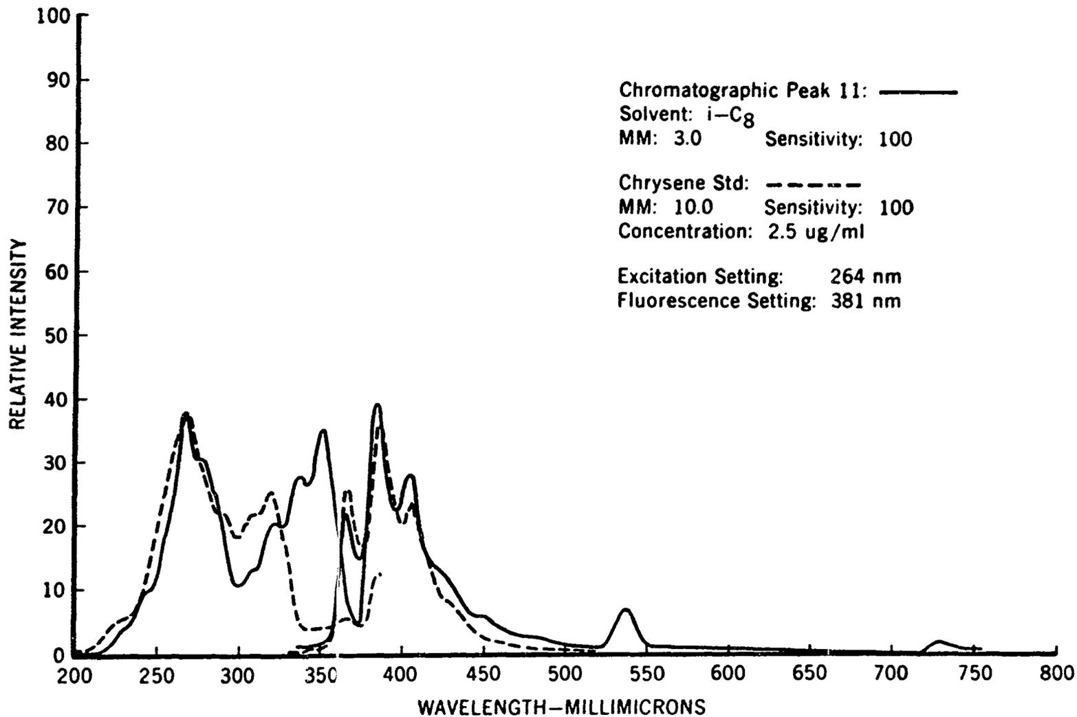
Figure 11.-- Excitation and Fluorescence Spectra of Chromatographic Peak 11 from SRF Carbon Black Extract and Chrysene.
