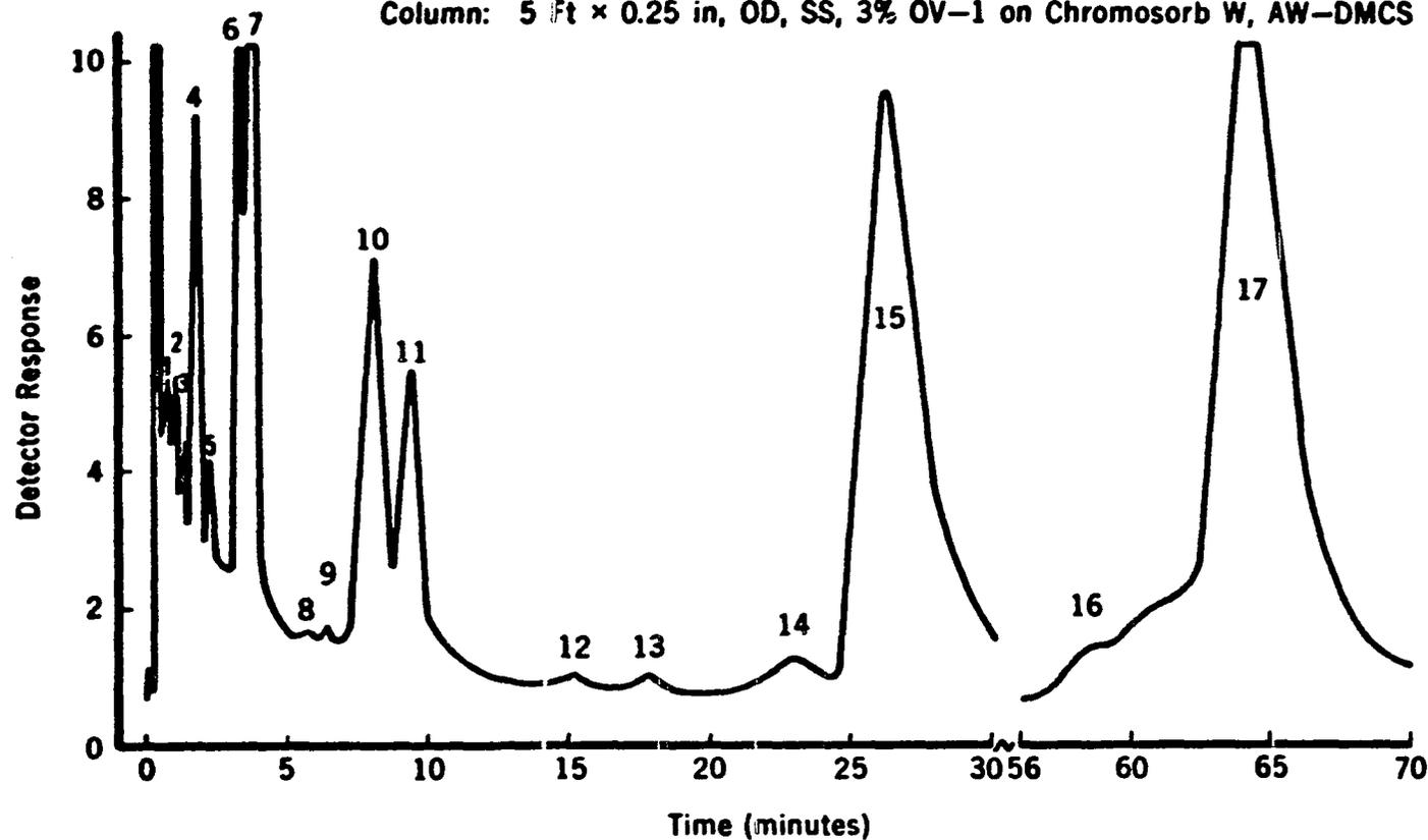
Figure 5.-- Gas Chromatogram of Polycyclic Aromatic Hydrocarbons from SRF Carbon Black with Flame Ionization Detector. Peak numbers corresponds to the compounds listed in table 9.
