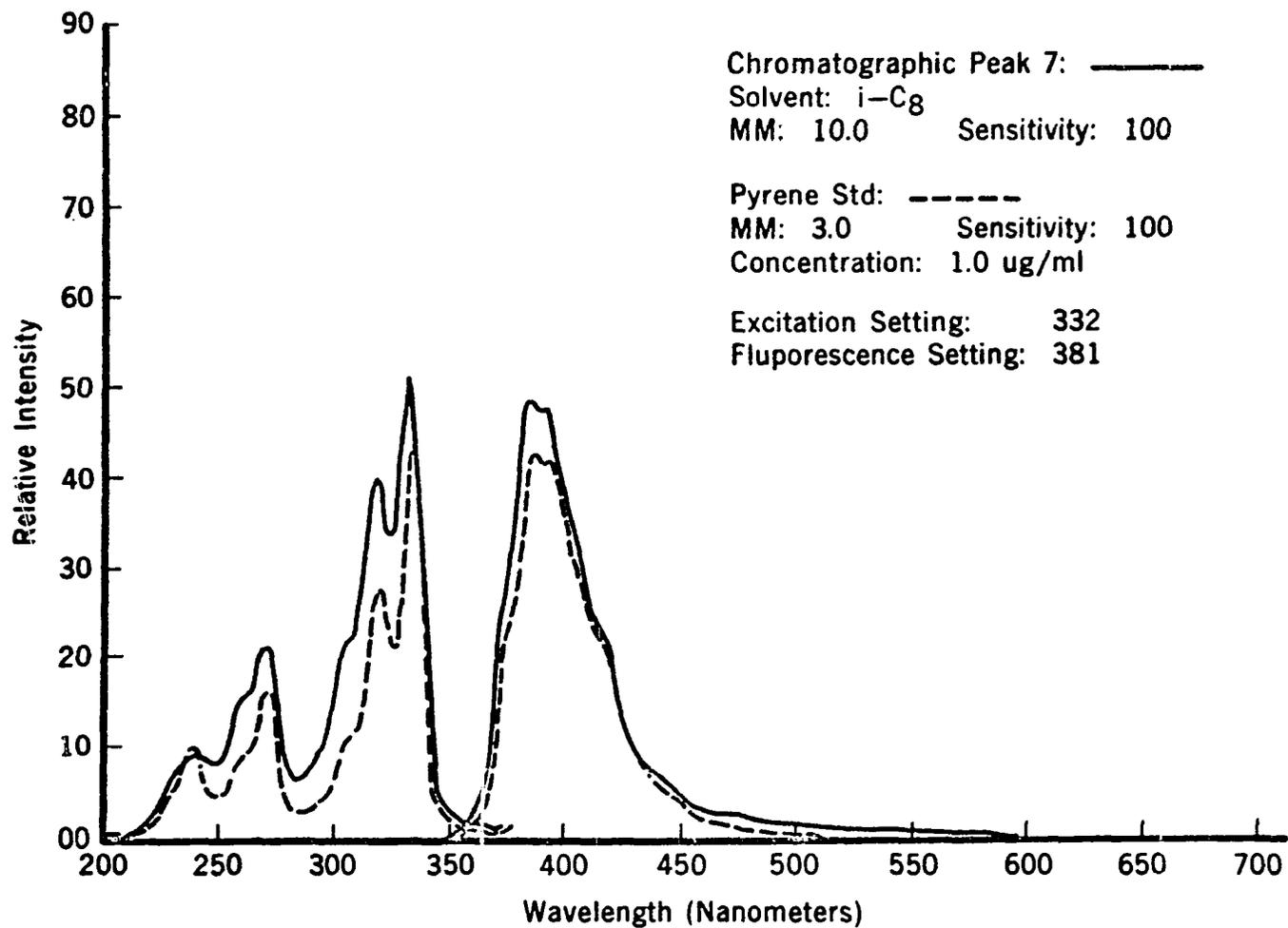
Excitation & Fluorescence Spectra of Chromatographic Peak 7 from SRF Carbon Black and Pyrene.
