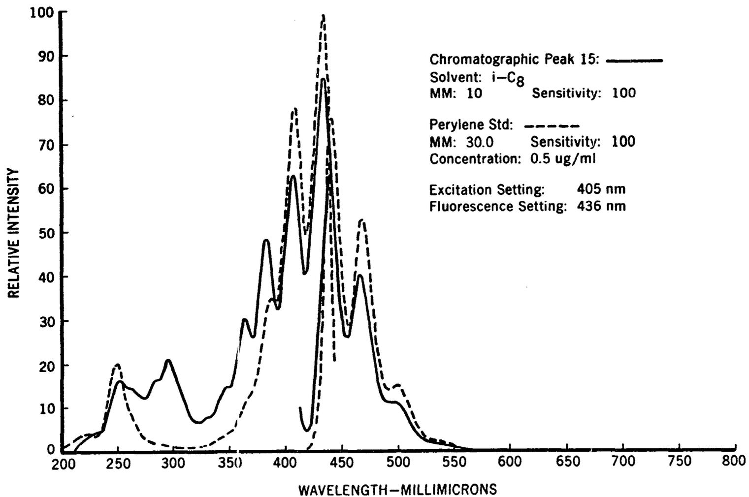
Figure 15.-- Excitation and Fluorescence Spectra of Chromatographic Peak 15 from SRF Carbon Black Extract and Perylene.
