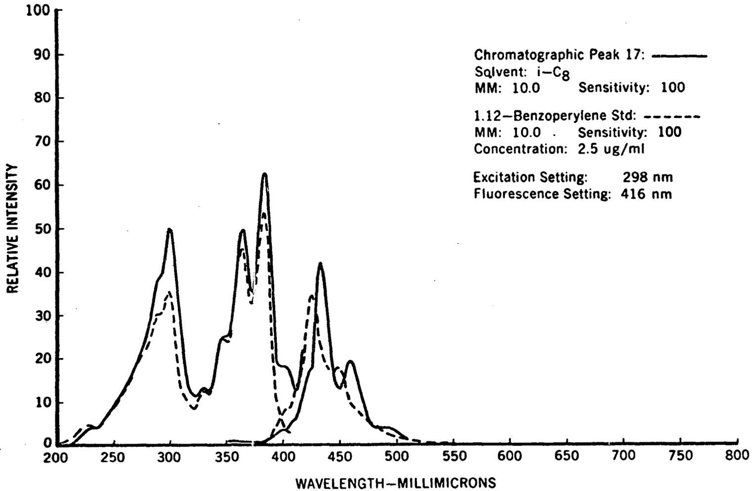
Figure 15.-- Excitation and Fluorescence Spectra of Chromatographic Peak 17 from SRF Carbon Black Extract and 1.12-benzoperylene.
