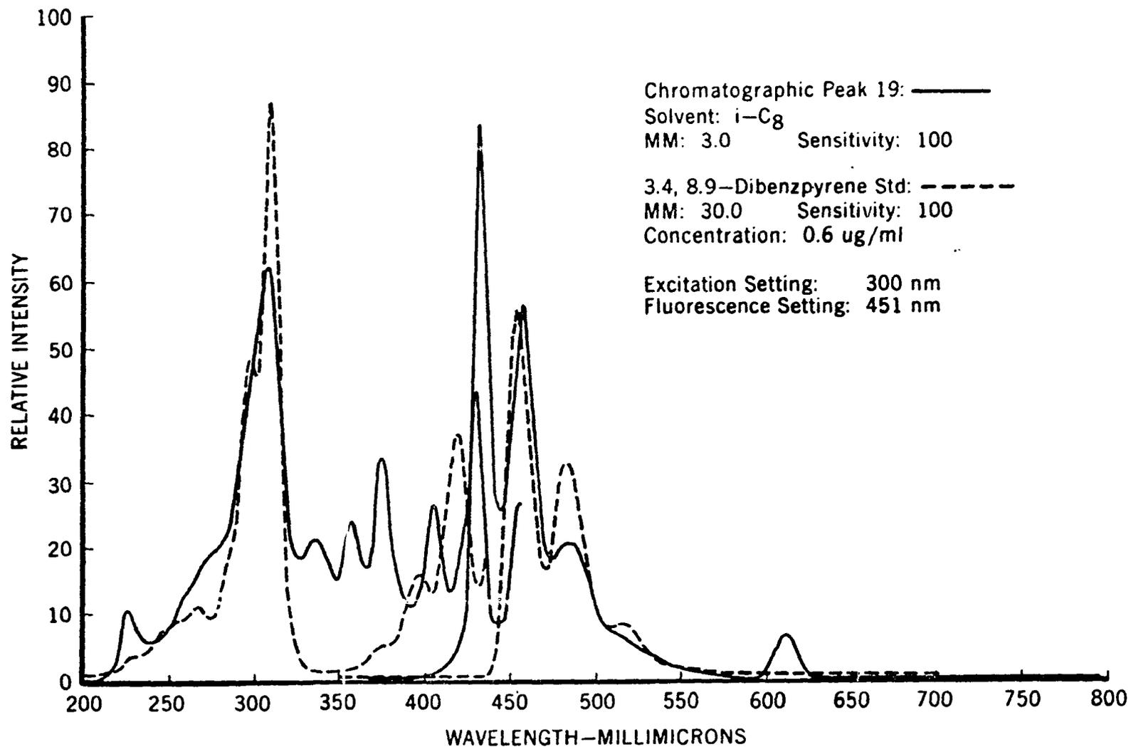
Excitation and Fluorescence Spectra of Chromatographic Peak 19 from SRF Carbon Black Extract and 3,4, 8,9-dibenzpyrene.
