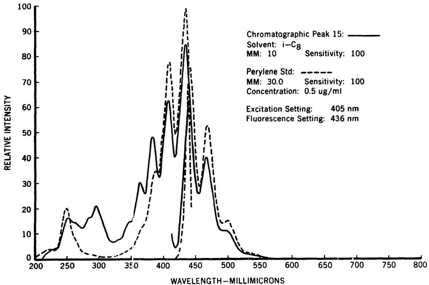
Excitation and Fluorescence Spectra of Chromatographic Peak 15 from SRF Carbon Black Extract and Perylene.
