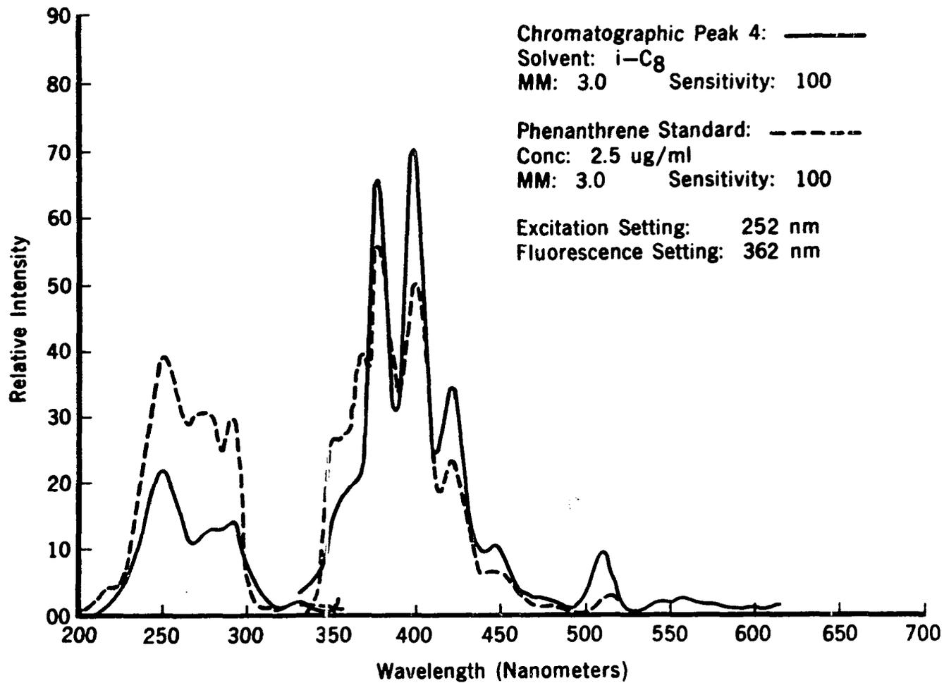
**Excitation & Fluorescence Spectra of Chromatographic Peak 4 and Phenanthrene in i-C<sub>8</sub>.**
