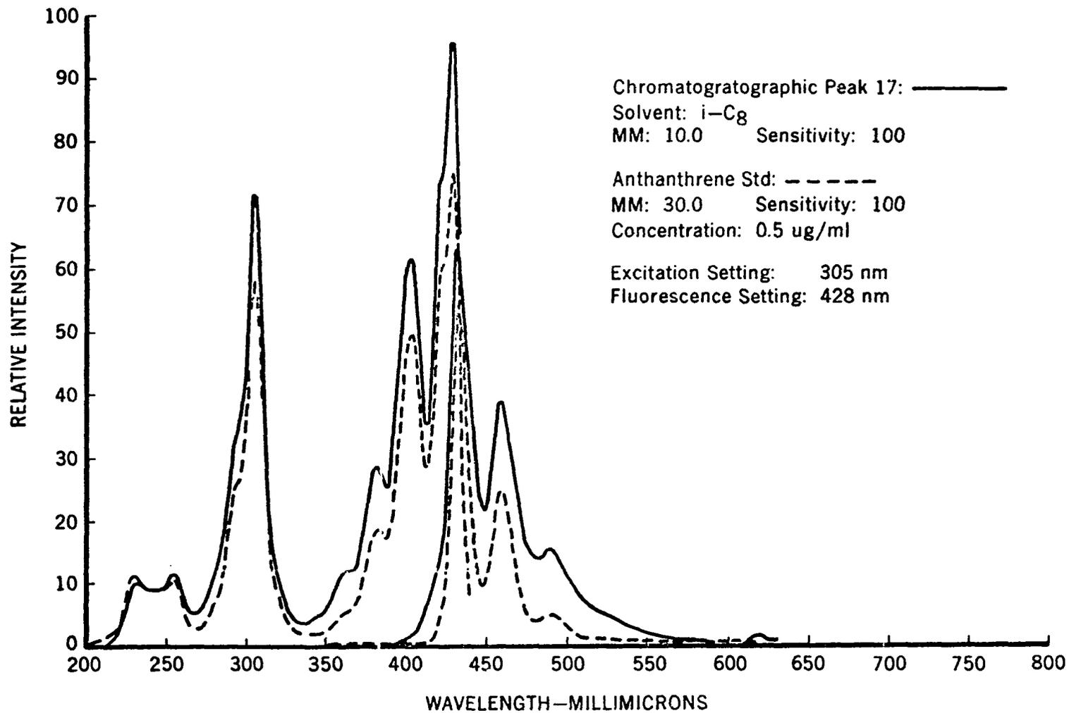
Figure 17.-- Excitation and Fluorescence Spectra of Chromatographic Peak 17 from SRF Carbon Black Extract and Anthanthrene.
