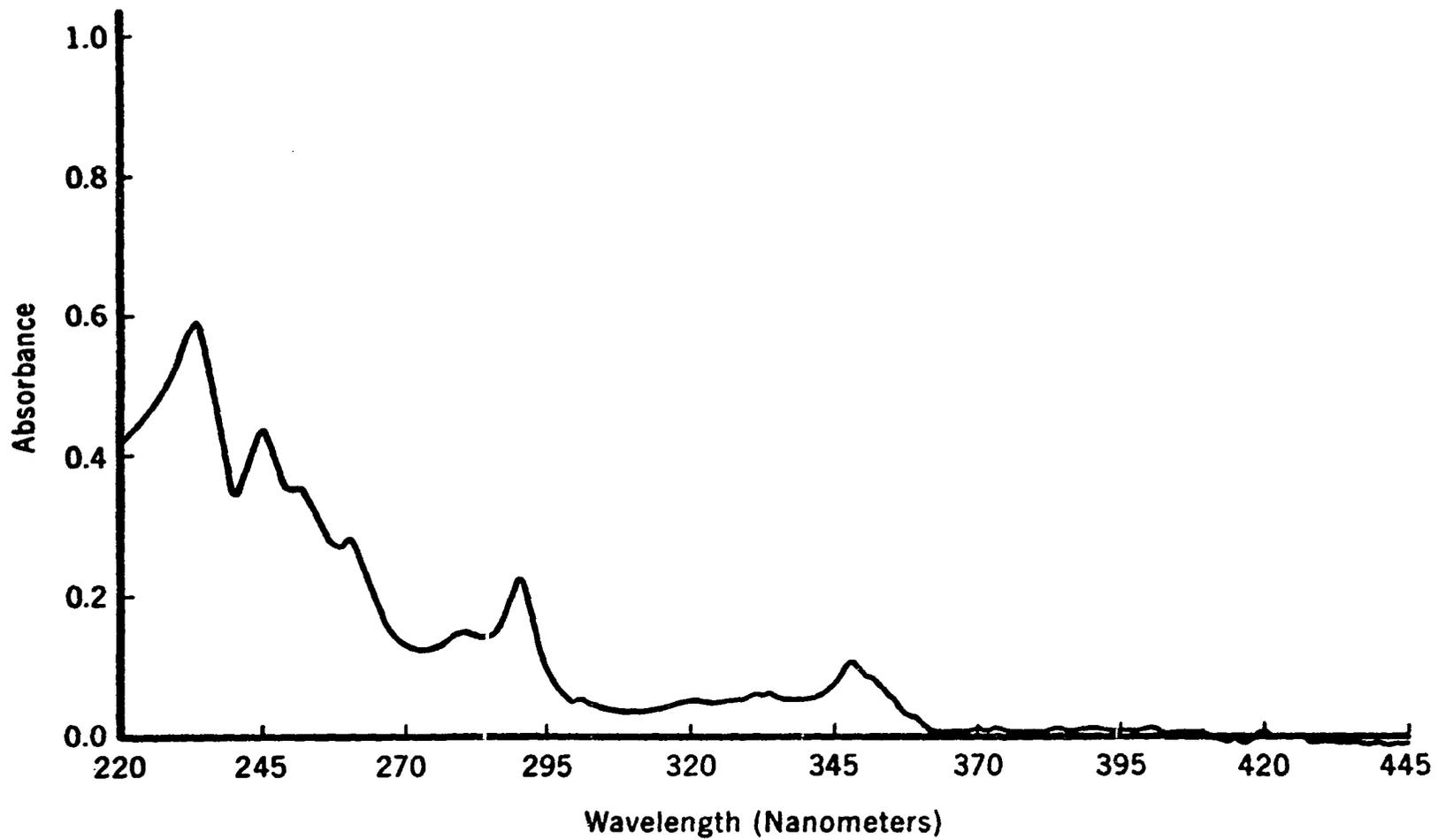
Figure 10.-- The Absorption Spectrum of Chromatographic Peak 10 in Iso-octane.
