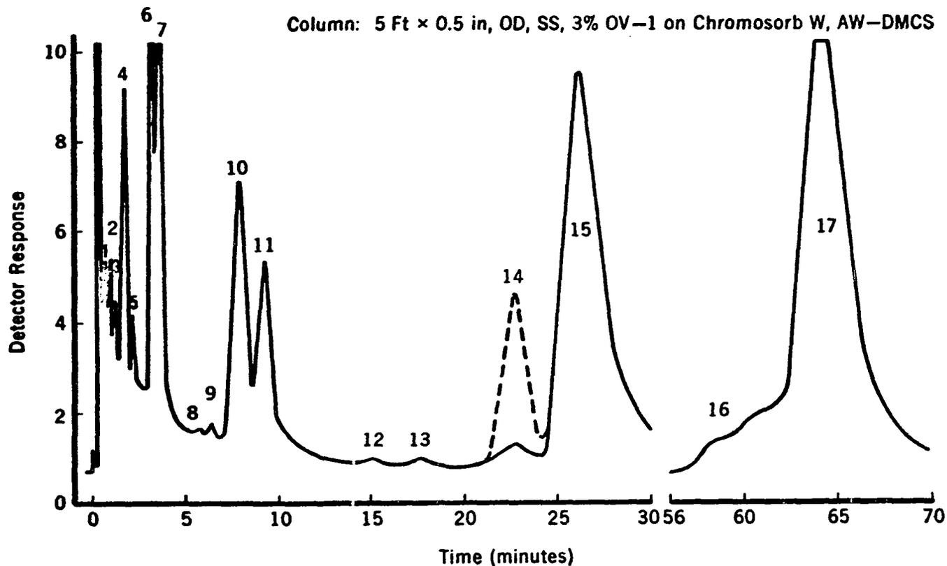
Figure 7.-- Identification of Chromatographic Peak 14 by Addition of a Suspected Compound (9, 10-dimethyl-1,2-benzanthracene).
