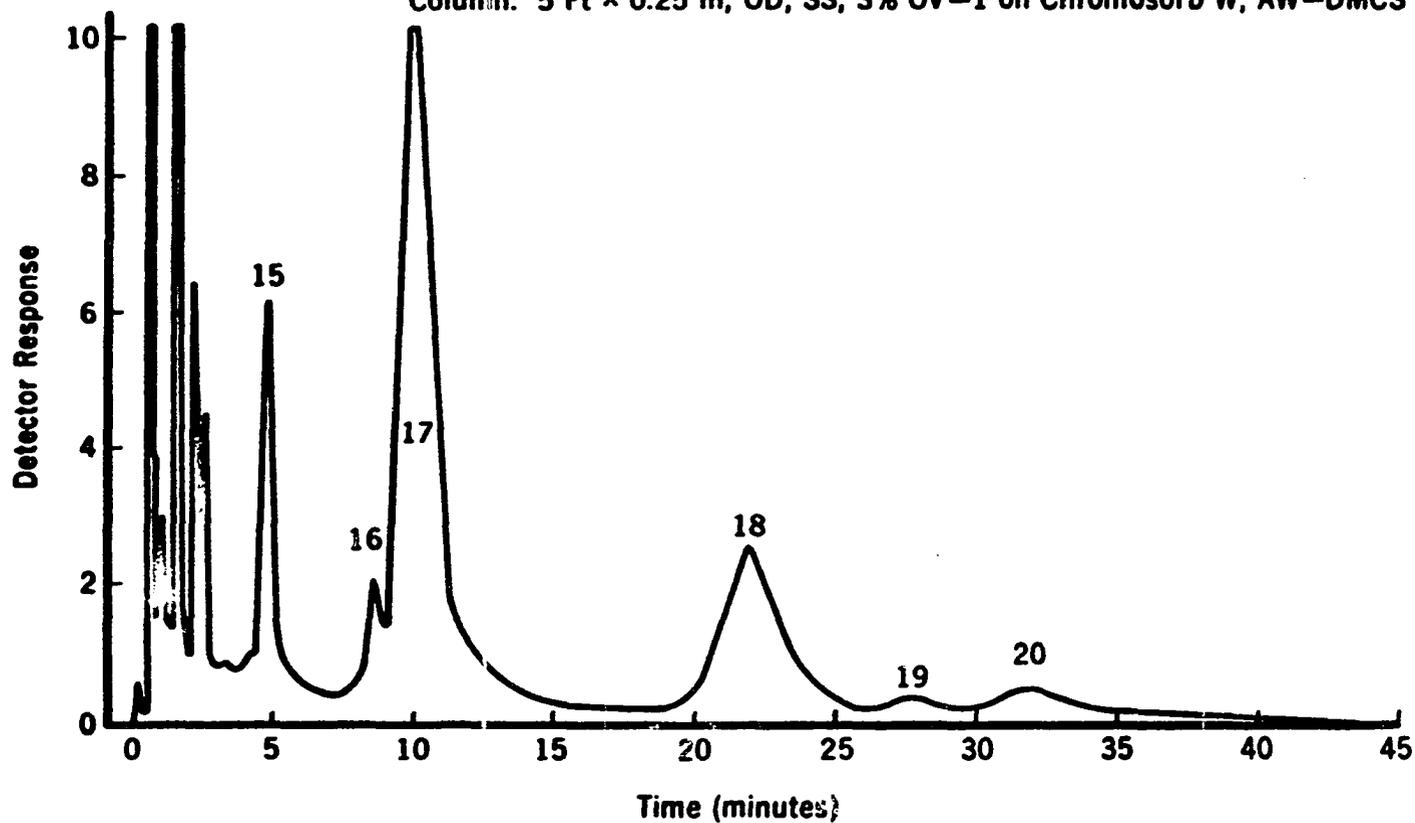
Figure 6.-- Gas Chromatogram of Polycyclic Aromatic Hydrocarbons from SRF Carbon Black.
