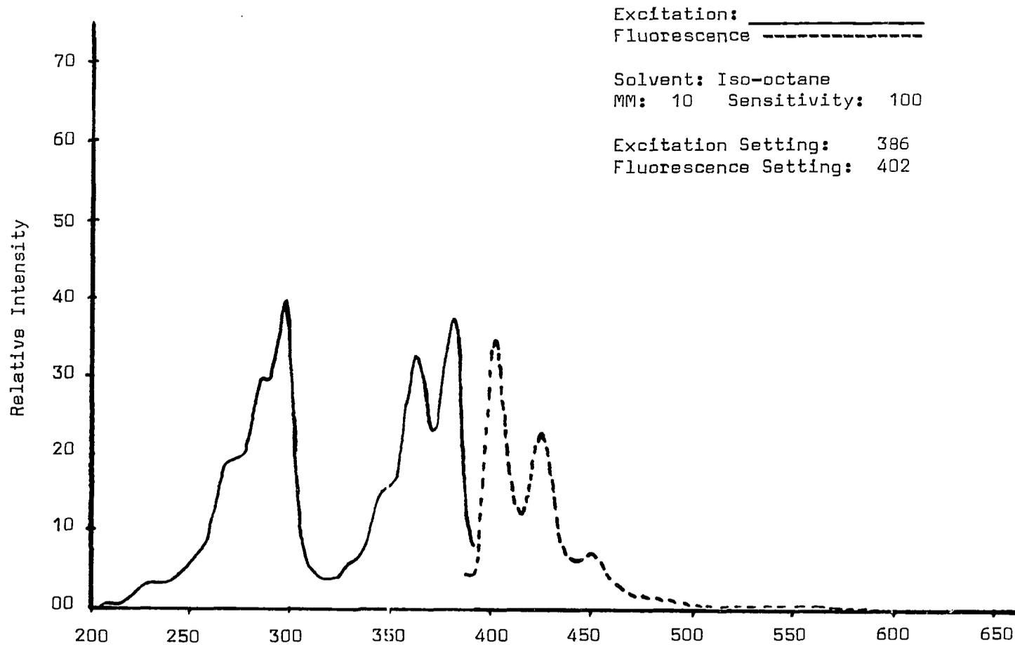
Figure 4.--Excitation and fluorescence spectra of BAP standard solution.
