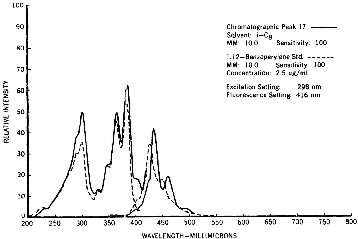
Excitation and Fluorescence Spectra of Chromatographic Peak 17 from SRF Carbon Black Extract and 1.12-benzoperylene.
