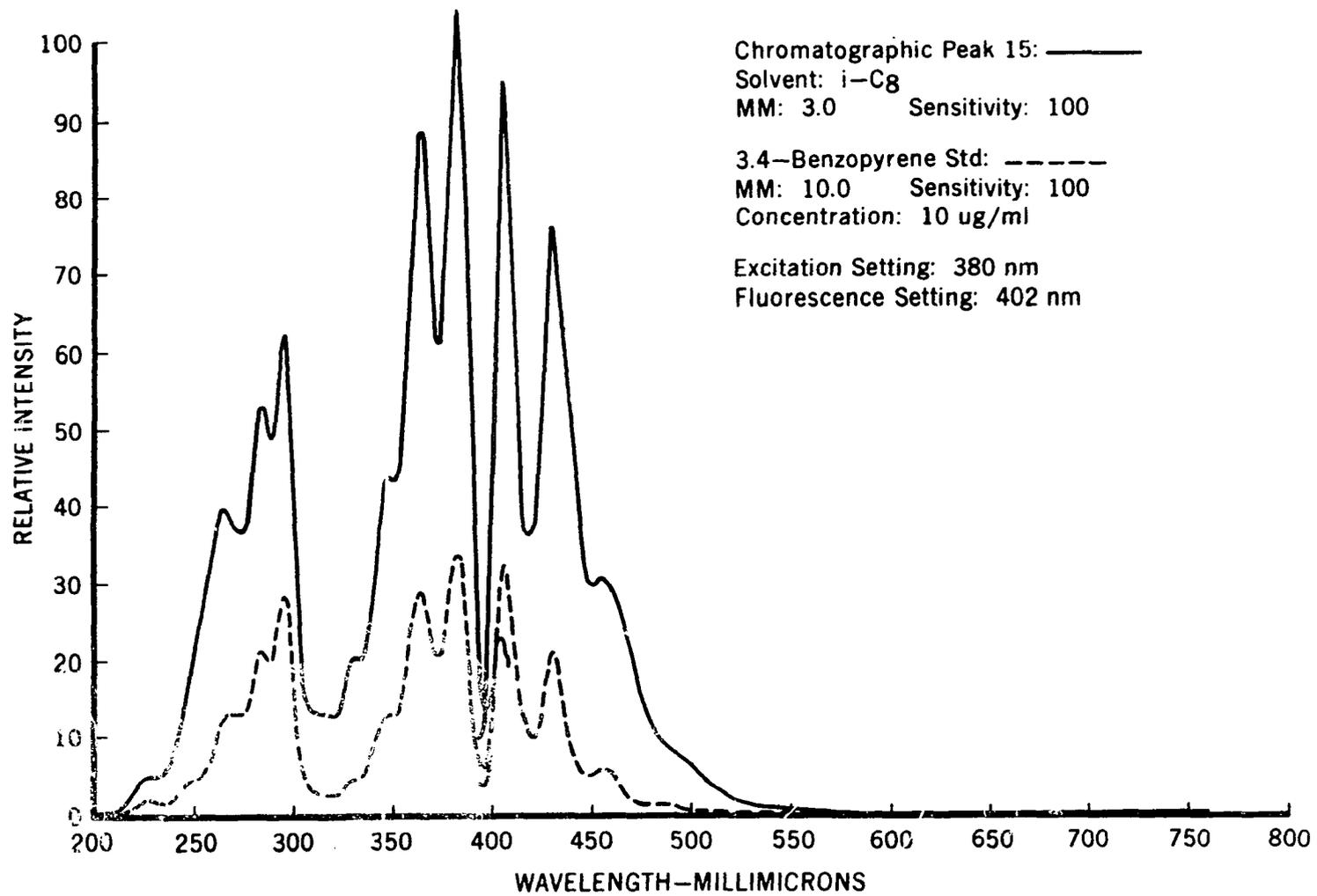
Excitation and Fluorescence Spectra of Chromatographic Peak 15 from SRF Carbon Black Extract and 3,4-benzopyrene.
