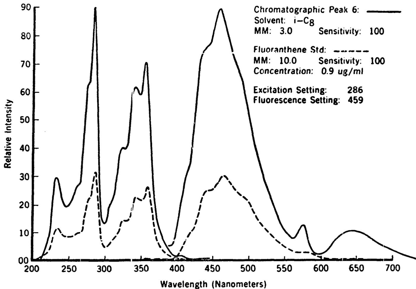
Excitation and Fluorescence Spectra of Chromatographic Peak 6 from SRF Carbon Black Extract and Fluoranthene.
