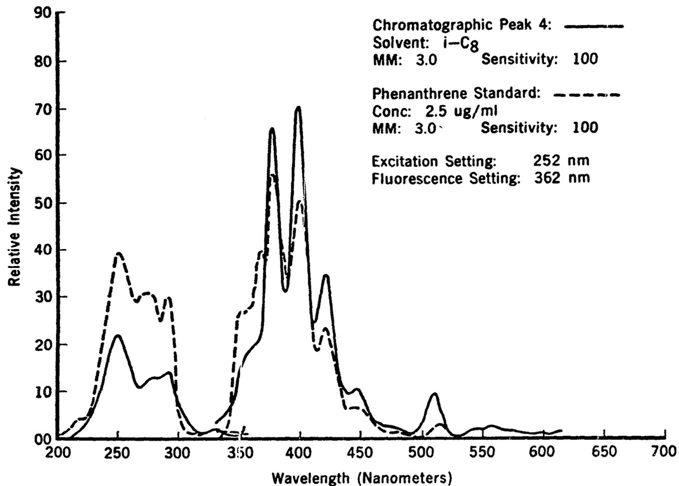
Figure 9. ---Excitation & Fluorescence Spectra of Chromatographic Peak 4 and Phenanthrene in i-Cg.
