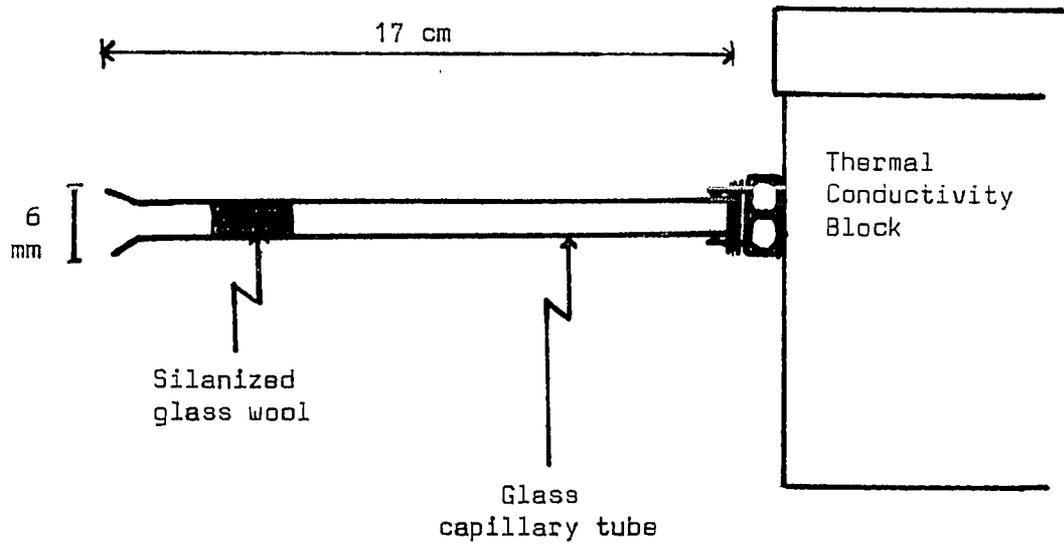
Figure 3.--Pyrex glass capillary tube for collection of chromatographic peaks.
