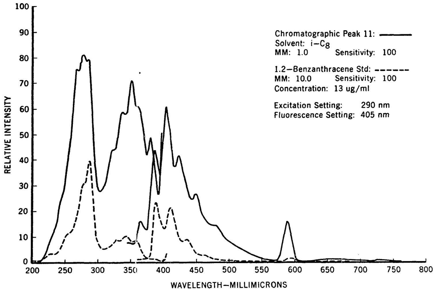
Figure 12.-- Excitation and Fluorescence Spectra of Chromatographic Peak 11 from SRF Carbon Black Extract and 1.2-benzanthracene.
