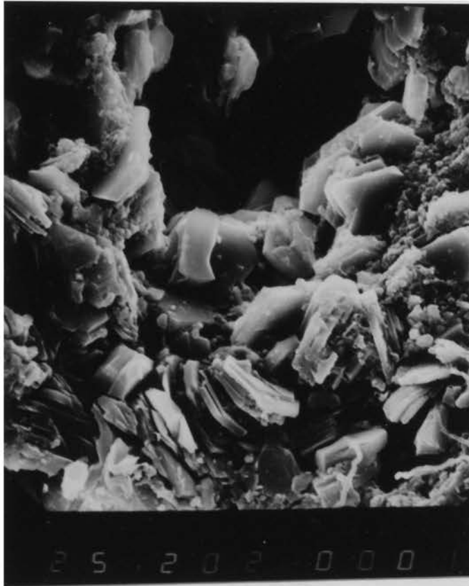
Figure 23. SEM Photograph of Stacked Pseudo-hexagonal Plates of Kaolinite Disrupted by Hematite in a Grape Creek Sandstone (X2000)
