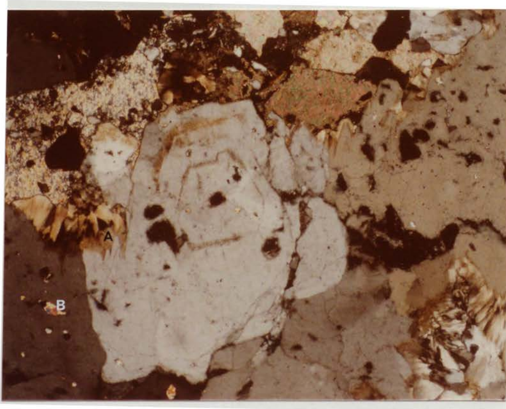
Figure 41. Photomicrograph of Megaquartz with Sequential Growth Rings (Note Multiple Dust Rims), Some of the Megaquartz Grades into a) Flamboyant Megaquartz; b) is Included with Anhydrite (X4, Crossed Nicols)
