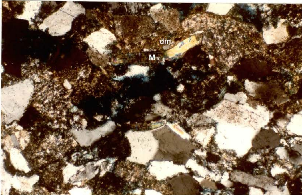
Figure 35. Photo-micrograph of Compaction Features; Broken Mica Grain and Squeezing of Detrital Mud Fragments, Lower Red Fork (Crossed Nichols)
