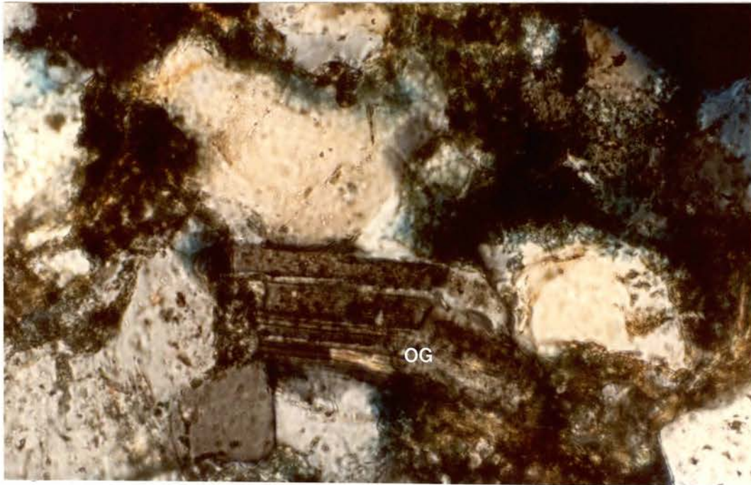
Figure 40. Photo-micrograph of Feldspar Overgrowths, Lower Red Fork (Crossed Nichols)
