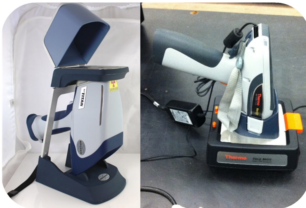
Figure 10: (Left) Bruker S1 Titan in Desktop Stand and (Right) Thermo Scientific Niton XL3t GOLDD+ in Field Stand
