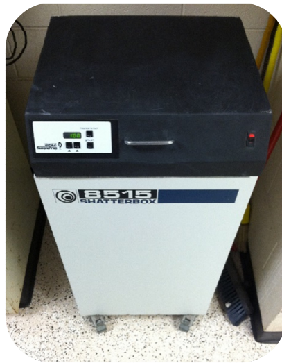
Figure 6: SPEX Shatterbox 8515 Used to Mill Samples
