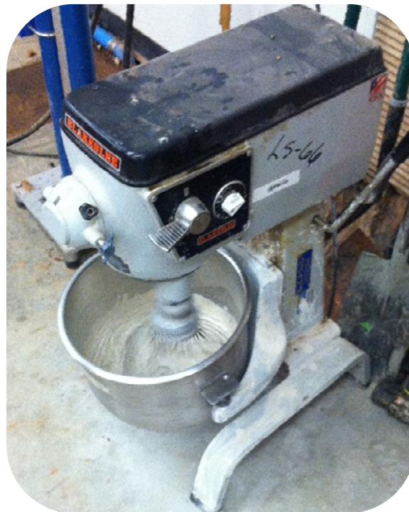
Figure 5: Mixing Samples with a Mechanical Blender
