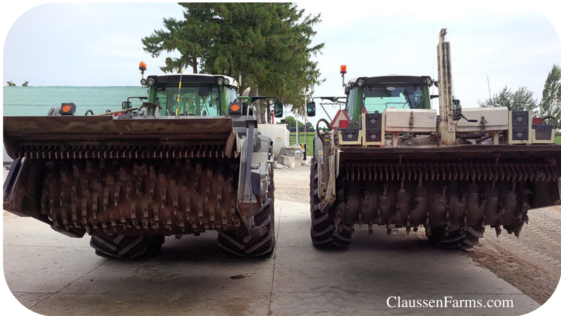
Figure 2: Self-Powered Mechanical Rotor Mixers
