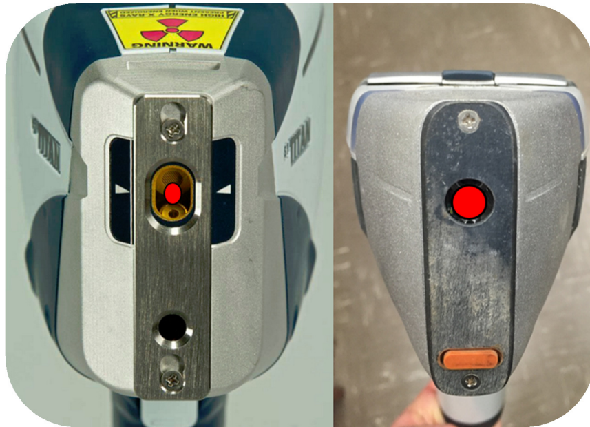
Figure 17: Beam Footprints of the S1 Titan (Left) and Niton XL3t (Right) PHXRF Devices
