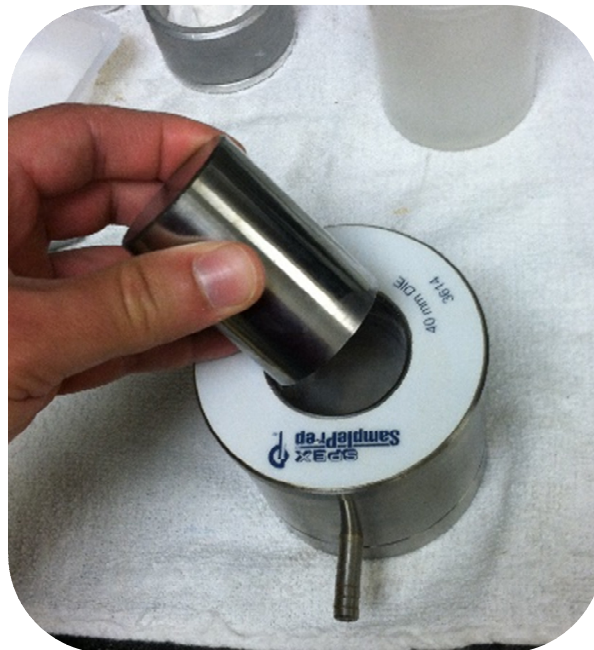
Figure 7: Removing Plunger from SPEX Evacuatable Die Set
