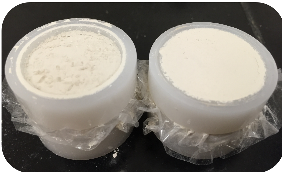
Figure 9: Poorly Prepared Powder Sample (Left) and Adequately Prepared Powder Sample (Right)
