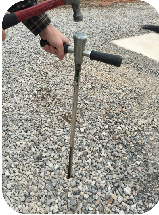
Figure 14: Hammer Head Soil Probe Used to Retrieve Samples at Various Depths
