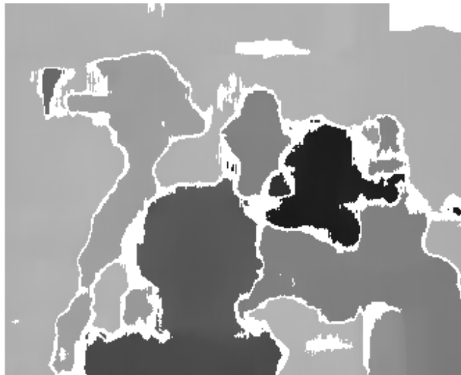
Figure 25. "Tsukuba" disparity map computed by the OpenCV block matching algorithm.
