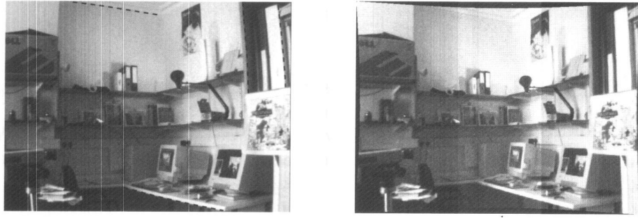
Figure 7. Lens distortion correction. Left: Original distorted image with dashed reference “straight” lines. Right: Distortion corrected image. ([10] fig. 7.6)
