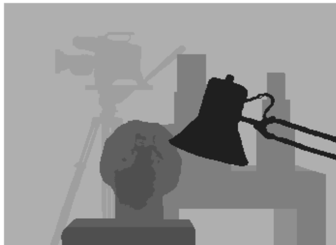
Figure 26. "Tsukuba" ground-truth disparity map. [17]
