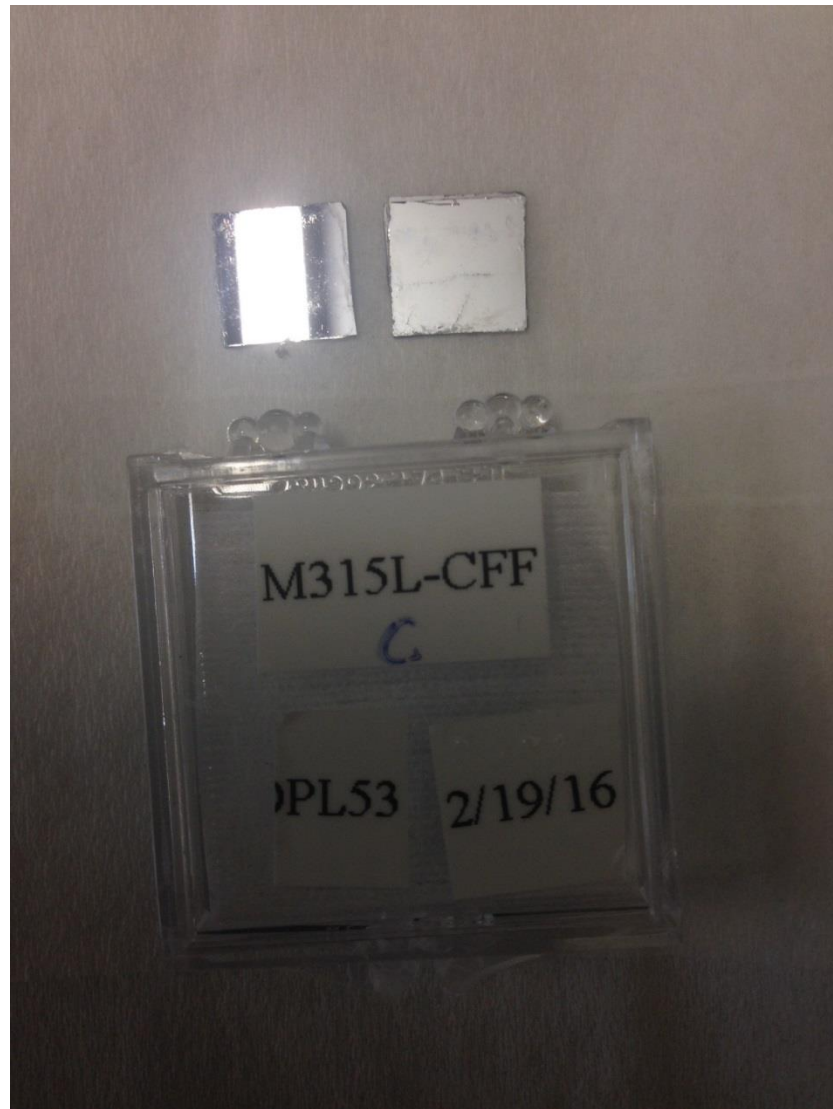
Figure 65 Image of M315 eutectic bonding to parylene-only bonded Si substrates after lift-off
