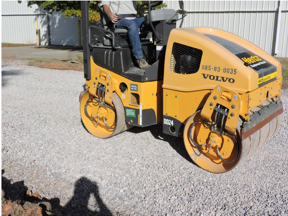
Figure 7.15 - 5 Ton Vibratory Compactor
