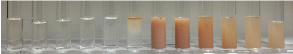
Figure 20: Pore Volumes collected from Column Study on CRA Sand with System 3 (0.94 wt.% Taiwan, and 1.1 wt.% NaCl)
