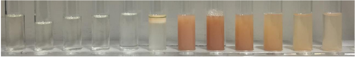
Figure 19: Pore Volumes collected from Column Study on CRA Sand with System 2 (0.75 wt.% AOT, 0.19 wt.% SDBS, and 0.7 wt.% NaCl)
