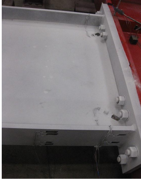
Figure 56. Jack's End-plate to Rafter Connection Prior to Testing
