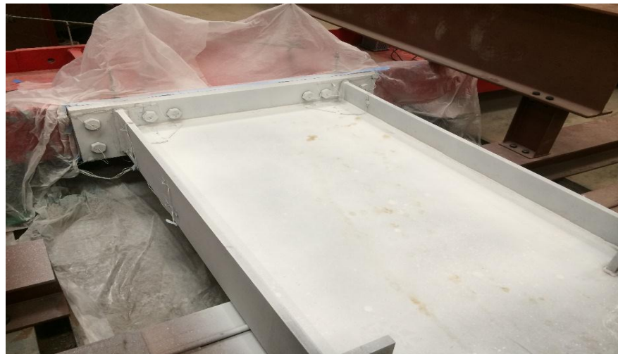
Figure 42. Test Specimen's Rafter with a Fresh Coat of White Wash
