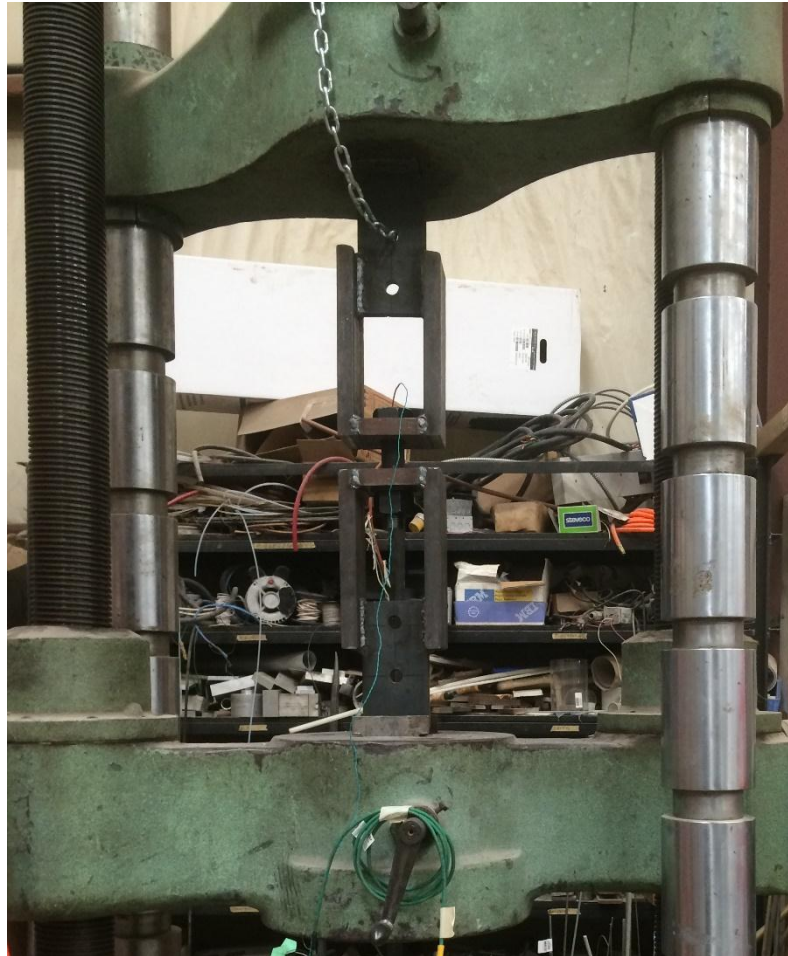
Figure 45. Bolt Being Calibrated
