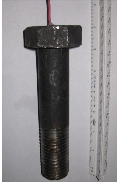
Figure 44. Fully Gauged Bolt
