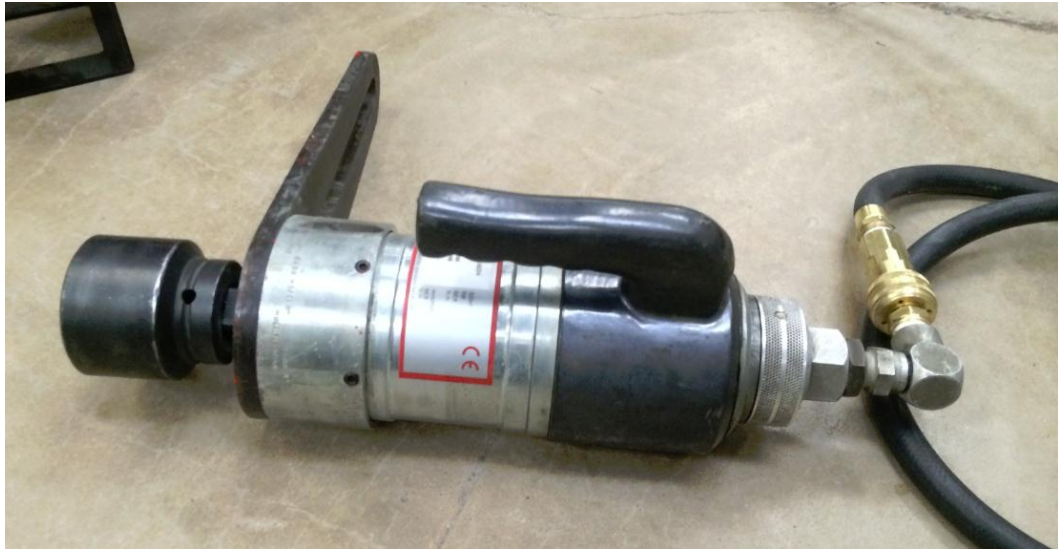
Figure 52. Norbar Pneutorque PT5, Pneumatic Torque Wrench
