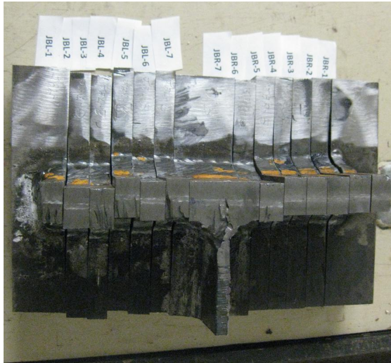
Figure 61. Cut Flange Specimens
