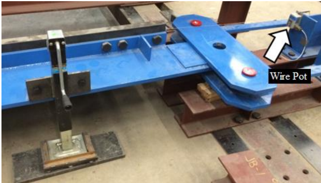
Figure 40. Wire Pot at Rafter's Tip
