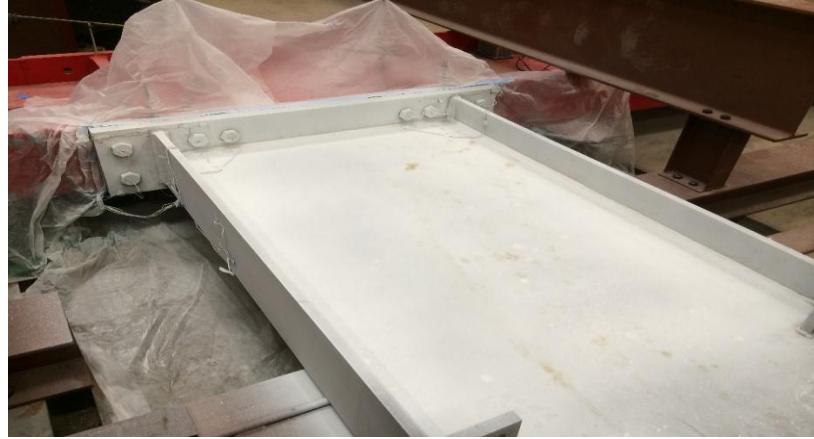
Figure 54. King's End-plate to Rafter Connection Prior to Testing
