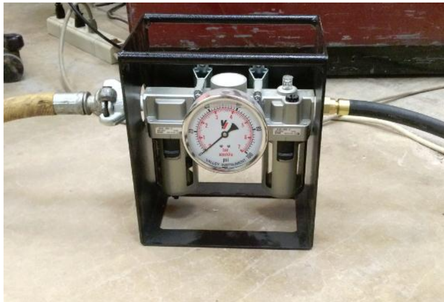
Figure 53. Pneumatic Torque Wrench Regulator
