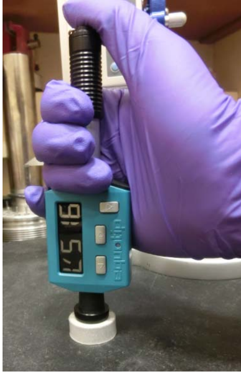
Figure 7. Rebound Reading on Berea Sandstone
