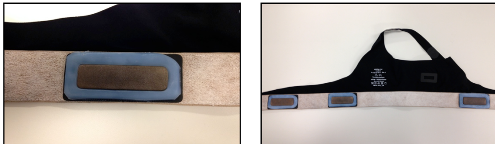
Figure 12. Silicone Putty Gaskets to Protect Electrodes
