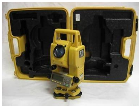
Figure 60: Total Station model Topcon GTS-211D used in this study to survey and monitor the deformations of GRS-IBS and conventional bridges in Kay County, OK
