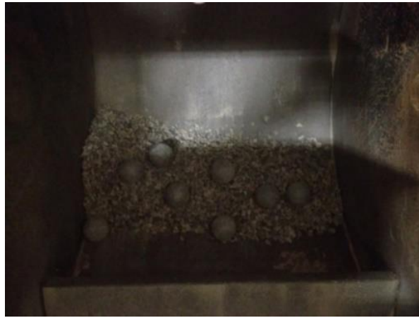
Figure 48: Test sample with eight steel spheres inside the L.A. Abrasion machine (Hatami et al. 2014)
