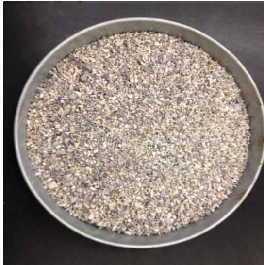
Figure 49: Oven-dried backfill sample retained on sieves Nos. 4 and 12 in Kay County (Hatami et al. 2014)
